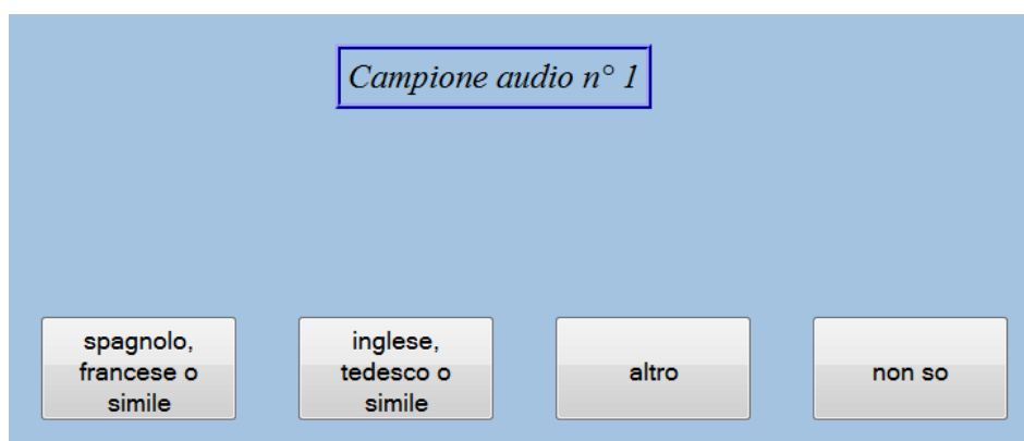
Figure 6.4. Screenshot of the interface. It consists merely of a label indicating the stimulus number and the four buttons. There is no button to listen to audio samples nor to proceed, as the succession of events is completely controlled by JavaScript.
