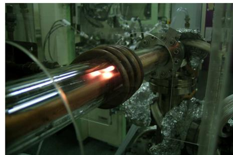
Figure 2.5: High temperature annealing of  $UCoGe$  for 12 hours just below the melting point ( $\sim 1350^\circ C$ ). The effect on the residual resistivity ratio is positive : the  $RRR$  increase from  $\sim 3$  to 30.
