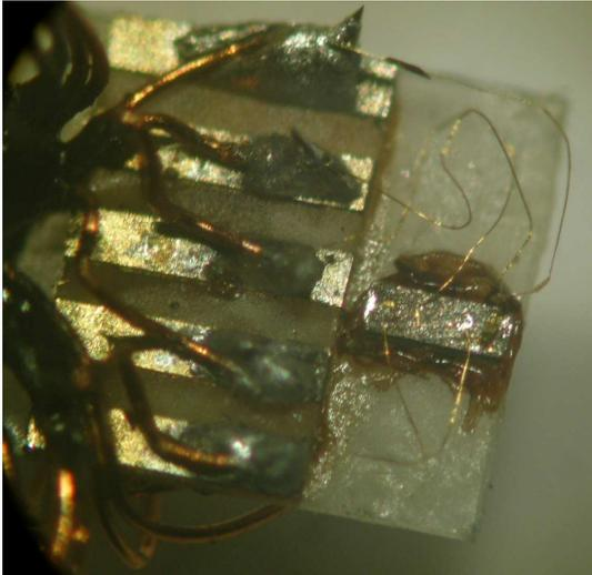
Figure 2.19: Experimental setup of the resistivity and AC calorimetry measurement under pressure on  $\text{UGe}_2$ .
