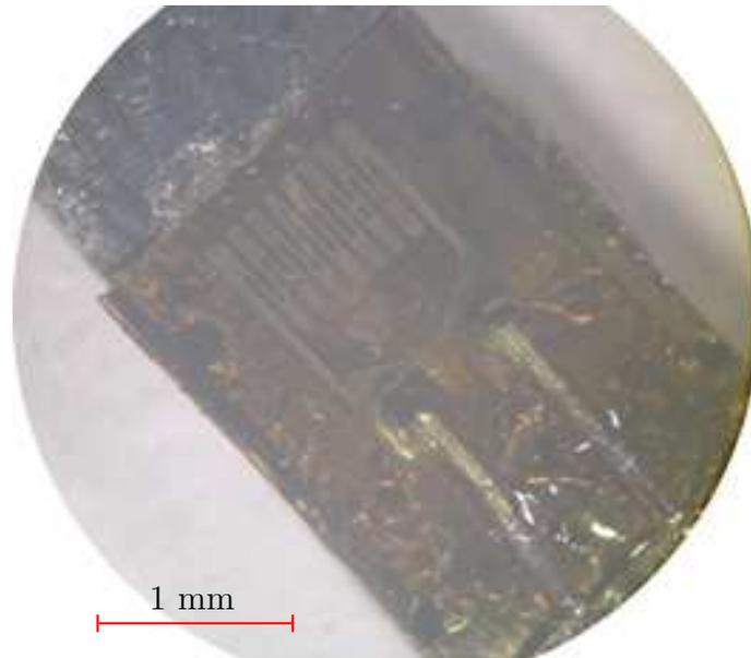
Figure 2.29: Commercial strain gauge glued on a sample of CeRhIn<sub>5</sub>.
