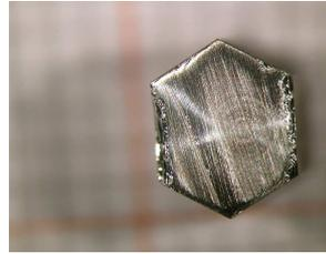
Figure 2.9:  $\text{URu}_2\text{Si}_2$  sample from growth #4. The left picture shows a  $c$  plane and the right one a polished  $a$  plane. This sample is prepared for an inelastic neutron scattering experiment under uniaxial pressure. The RRR is around 20 which is not very good for this material, but the rocking curve revealed only one grain, which is remarkable for such a big sample.
