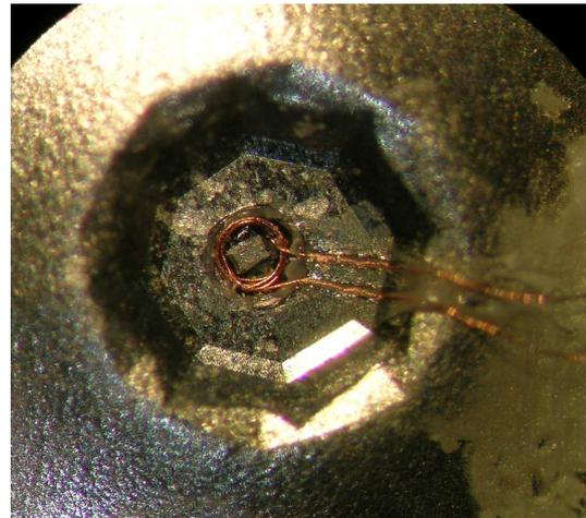
Figure 2.16: Inside view of the diamond anvil cell for AC susceptibility measurement on  $\text{UGe}_2$ . In addition to the ruby, a small piece of tin (Sn) has been used to determine the pressure. The homemade pick-up coil consists of 10 loops of copper wire whose diameter is  $14\ \mu\text{m}$ . The excitation coil (not visible here) is outside the pressure chamber.
