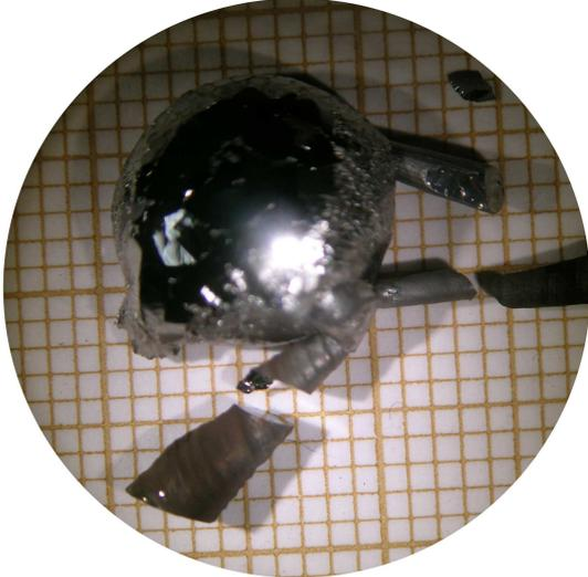
Figure 2.38: As grown  $\text{URu}_2(\text{Si}_{1-x}\text{Ge}_x)_2$  with  $x \approx 9\%$ . During the pulling of the single crystal, the ingot accidentally dropped down and melt again (spherical polycrystal in the picture), but the arc discharges have been stopped almost instantaneously so that pieces of single crystals remain.
