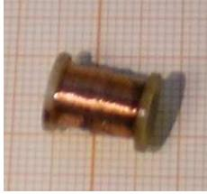
Figure 2.35: Excitation coil for AC susceptibility measurements in a He<sup>3</sup> PPMS refrigerator.
