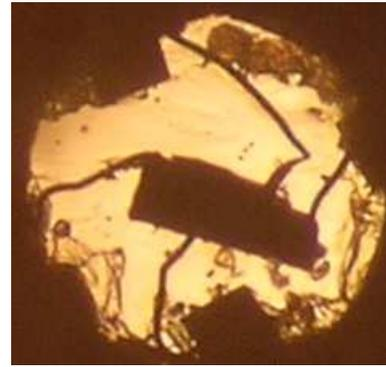
Figure 2.14: Inside view of the diamond anvil cell for resistivity measurement on  $\text{UGe}_2$ . The gold wires (diameter  $10\ \mu\text{m}$ ) are spot welded on the sample on one side, and squeezed on flattened gold wire (initial diameter  $25\ \mu\text{m}$ ) going through the gasket.
