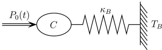
Figure 2.17: Simplified model for the AC calorimetry. The sample with a specific heat  $C$  is coupled to a thermal bath at the temperature  $T_B$  through a thermal leak of conductivity  $\kappa_B$ .
