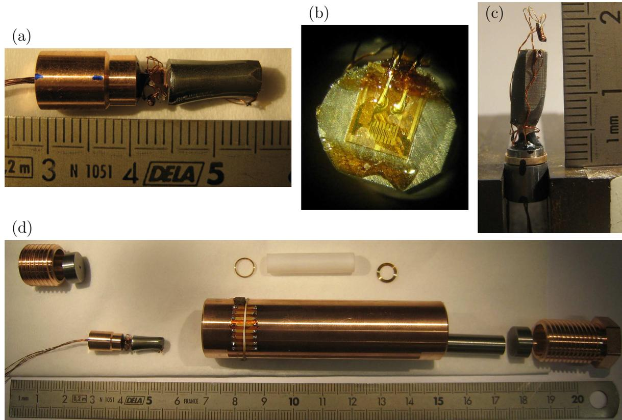
Figure 2.33: Experimental set up of two obturators (a) and (c) for two similar pressure cells (d). The big samples are single crystals of  $\text{URu}_2\text{Si}_2$ . A strain gauge is glued on top of each sample for thermal expansion measurement (b). A home-made Pb-manometer is used to determine the pressure.
