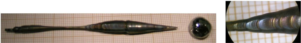
Figure 2.37: As grown ingots of URu<sub>2</sub>Si<sub>2</sub> #G4 in a tetra arc furnace using a seed oriented along the  $a$ -axis. The  $c$  plateau can clearly be observed.
