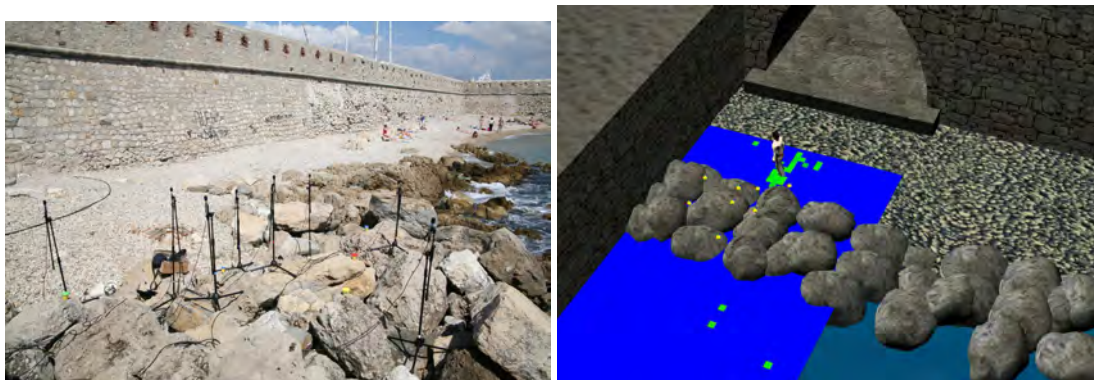
Figure 6.5: Left: Recording setup used for the seashore recordings. Right: Example virtual reconstruction of a seashore with walking pedestrian. Yellow spheres correspond to the locations of the microphones used for recording.
