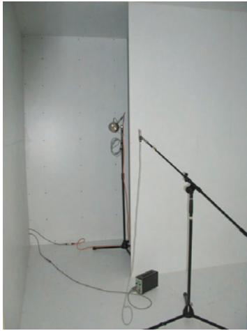
2 We can mount additional panels inside the Bell Labs Box to study the effects of sound diffraction.
