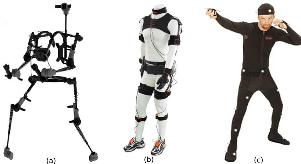
FIGURE 2.1: Examples of systems using markers. (a) exoskeleton of *Gypsy*<sup>™</sup> mechanical system. (b) markers of *Xsens*<sup>™</sup> inertial system. (c) markers of *OptiTrack*<sup>™</sup> passive optical system.
