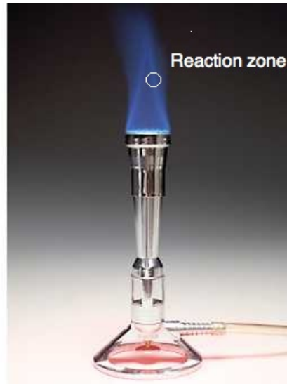
Figure 2.9: Picture showing premixed flame from a Bunsen burner. The small white circle denotes a portion of reaction layer on the flame surface.
