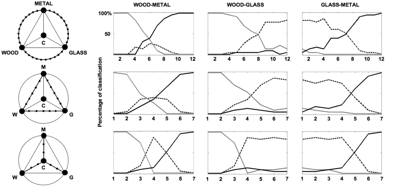
Fig. 8. Perceptual evaluation test of the control strategy. Left: position of sounds (black markers) used for the test in the Material Space as a function of the trajectory: along the external circle (first row), along the chords whose endpoints are the reference sounds (second row) and along the radii of the circle from the center C to the reference sounds (third row). Right: percentage of classification as Wood (gray curves), Metal (black curves), or Glass (dashed curves) corresponding to the three types of trajectory for each sound as a function of its position of the continuum.
