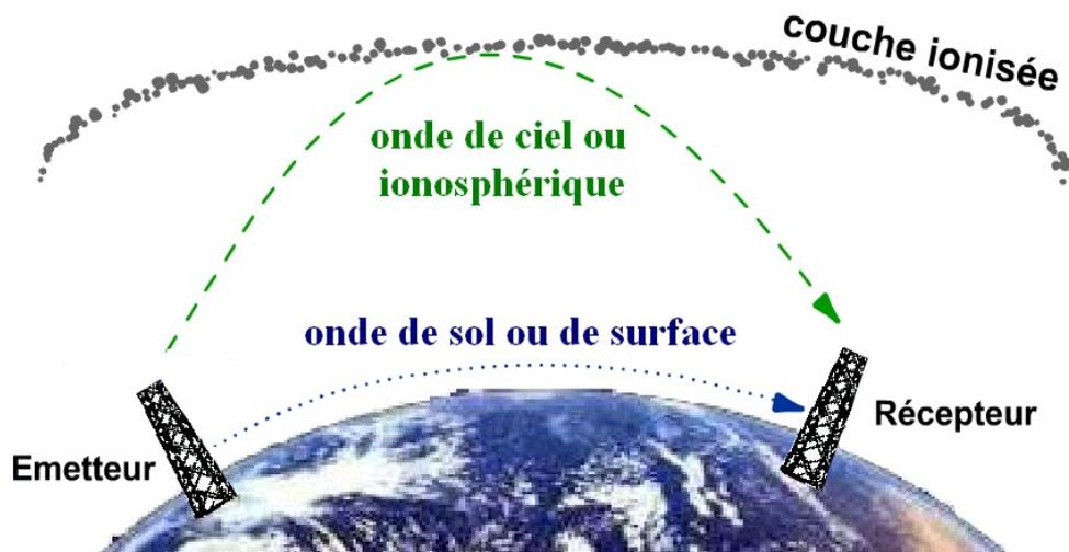
Figure I.1 Propagations VLF/LF
