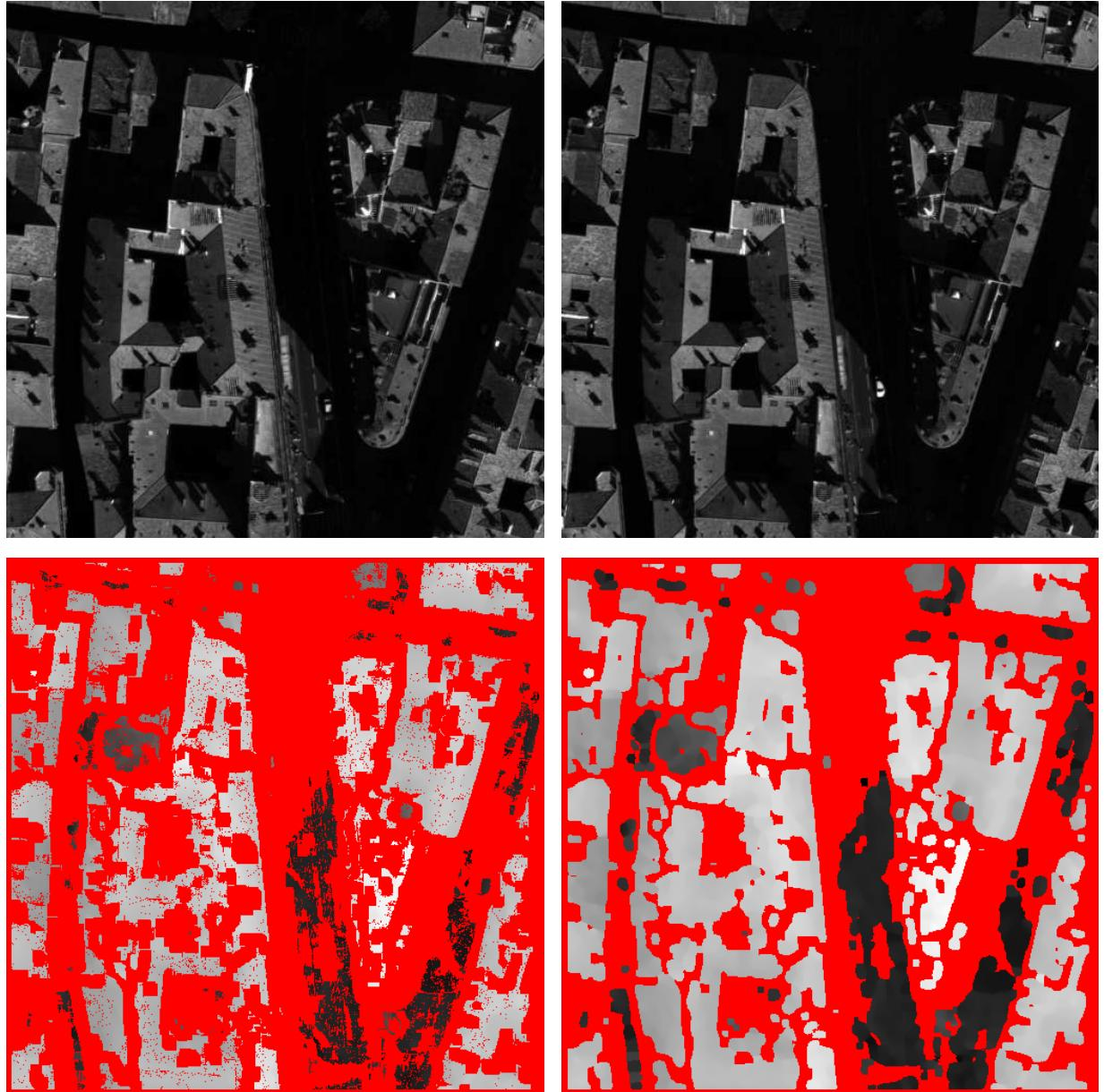
Figure 6.13: “Esquirol neighborhood” (Toulouse). Top: pair of stereo images with 20cm resolution and  $B/H = 0.08$ . Bottom: on the left, disparity map. The disparity map is not very dense (32%) because of the numerous shadows. Moreover, houses with different heights are right next to the others, and several patches are rejected because they risk fattening. The moving car has not been matched. On the right, disparity map after median filter (51% density).
