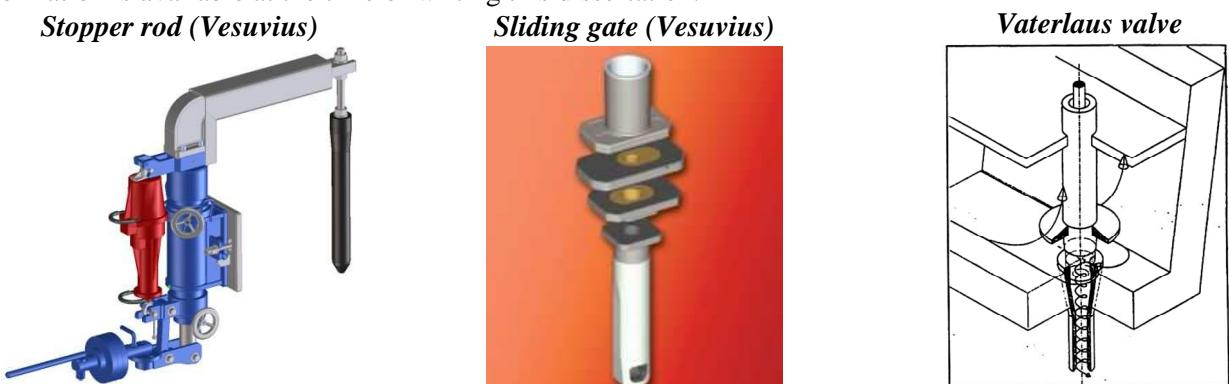
Fig. 1.32. Types of flow control valves
