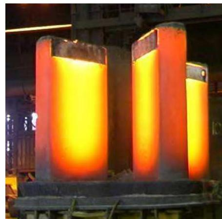
Fig. 1.17. Ingots solidification in progress
