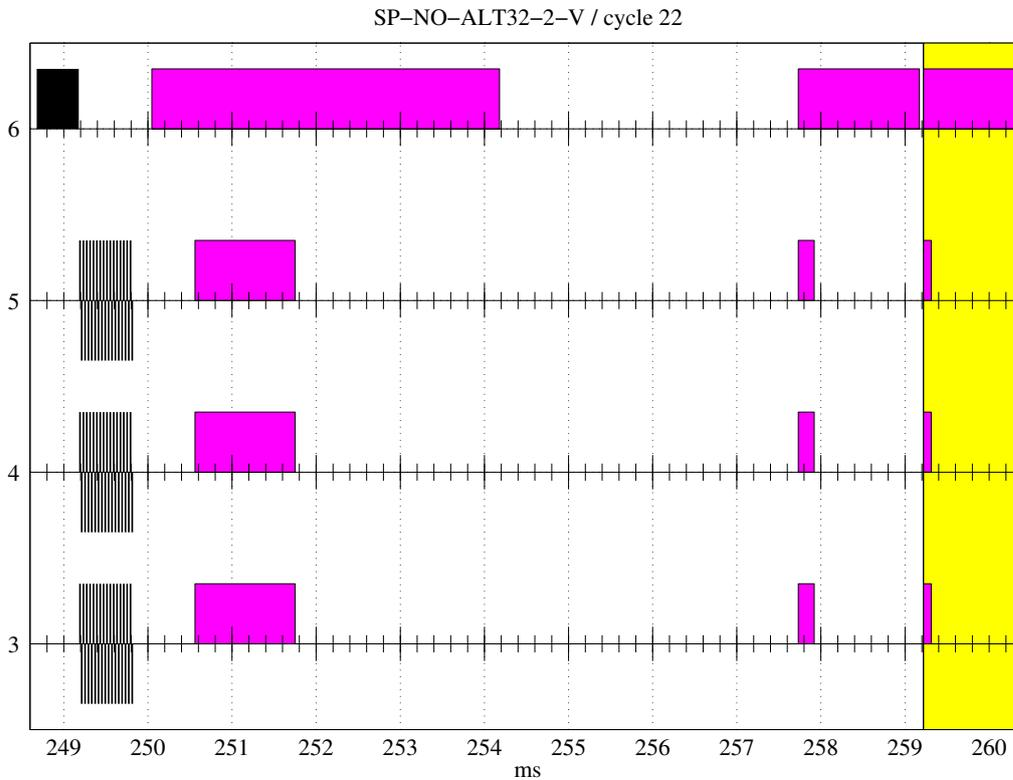
Figure 2.7: Time diagram of the pulsing of the 22<sup>nd</sup> cycle of the 32 bits strong condition alternating code of ALT-32-2-V . *black* is for the transmitted pulses, *dark gray* is for the receiving periods and *light gray* is when the calibrated noise source is injected. The background and calibration measurements are performed at the end of each cycle. The whole 64 cycles are run in 764 ms and have been optimised for a 10 s pre-integration time
