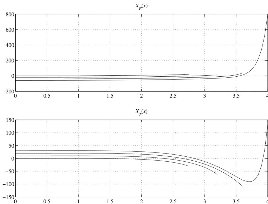
Figure 4.1: The  $X_E$  and  $X_T$  functions for different values of the upper boundary of integration  $x_{\max} = v/v_e\sqrt{2}e = 2.8, 3.2, 3.6$  and  $4.0$ , and for an ion charge number  $Z=1$ . The  $X_E$ 's are shifted by  $-20$  with each other, the  $X_T$ 's are shifted by  $+10$  with each other, the reference curves (i.e. not shifted) are for  $x_{\max} = 2.8$
