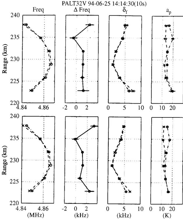
**Fig. 5.** The fitted parameters  $f_r$ ,  $\Delta f_r$ ,  $\delta_f$  and  $a_p$  as well as the error bars from the data of Fig. 4 as a function of range. The *dashdot* line is for the parameters from the upshifted line, and the *dashed* one is for the downshifted lines. The four upper panels show the parameters for the squared-triangle model, the four lower panels for the Gaussian model
