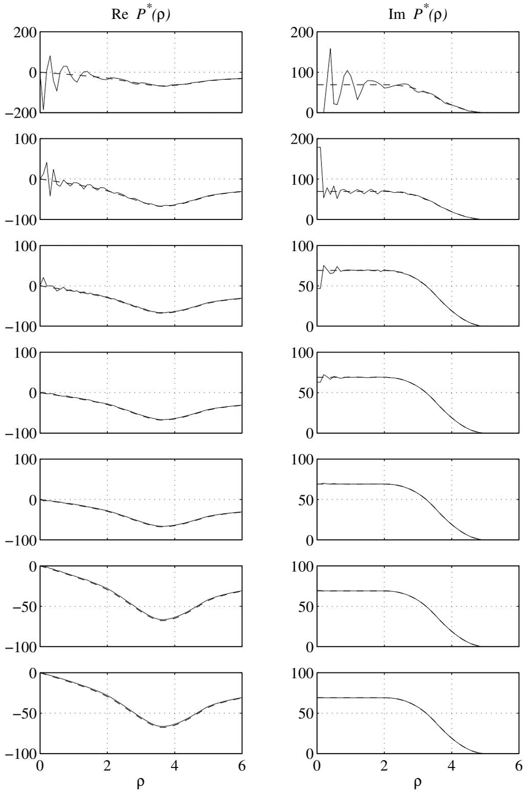
Figure 1.5: Test of the  $P^*$  function, for  $\rho \geq 0$ , with the triangle function of parameters  $a = 2$  and  $h = 3$ . From top to bottom the number of points in the quadrature are 16, 32, 64, 128, 256, 512 and 1024. The *dashed* lines are for the analytic expressions of Eqs. (1.47) and (1.48). The *solid* lines are for the numerical calculations with our code
