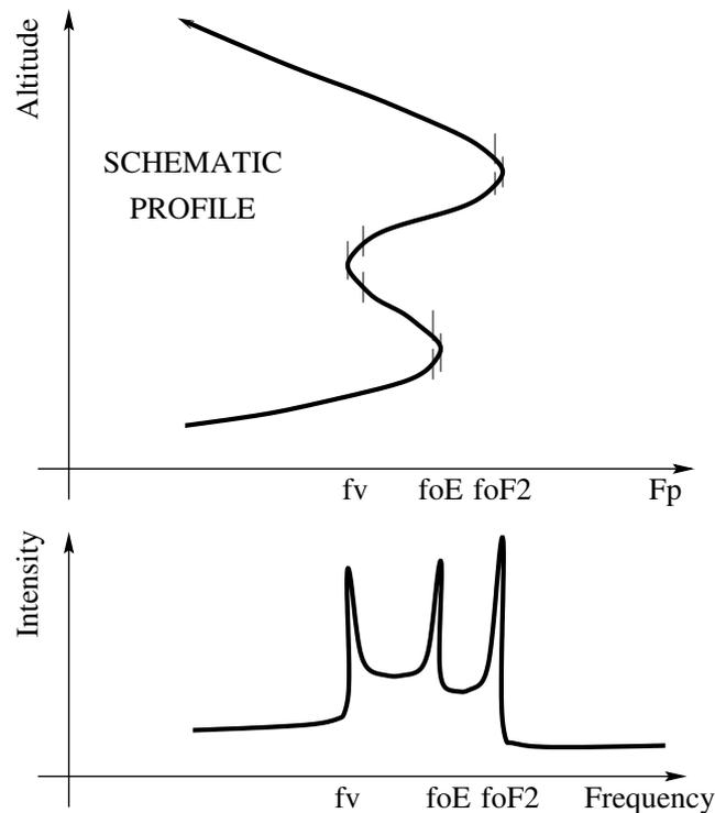
Figure 2.2: Principle of the long pulse measurement of the plasma lines. The critical frequencies  $f_v$ ,  $f_oE$  and  $f_oF2$  can be estimated by locating the abrupt signal drop in the power spectrum
