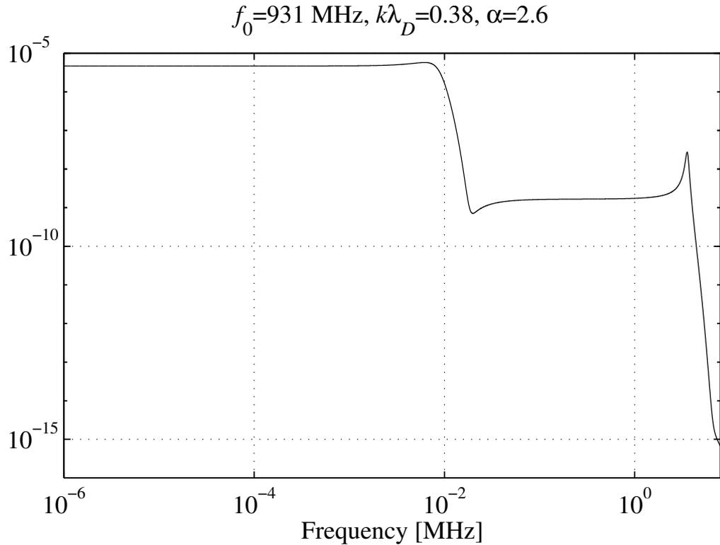
Figure 1.3: Theoretical incoherent scatter spectrum for the UHF EISCAT radar (931 MHz) for a Maxwellian plasma with the same ionospheric parameters as in Figure 1.2 and using the differential cross section model of Eqs. (1.7)–(1.14)
