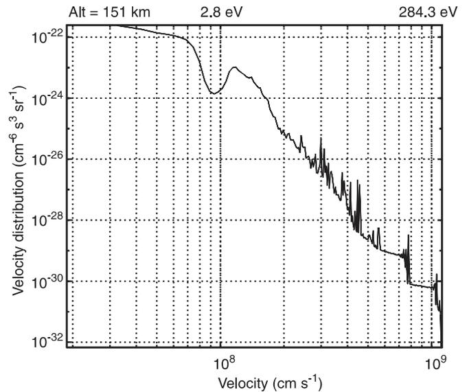
**Fig. 2.** The suprathermal angular velocity distribution function calculated by the transport code for an eight-stream calculation at 151 km and for a pitch angle of  $86^\circ$  (i.e.  $\mu=0.0694$ ). The distribution is nearly isotropic, and the data at other pitch angles would not be distinguishable on the same plate
