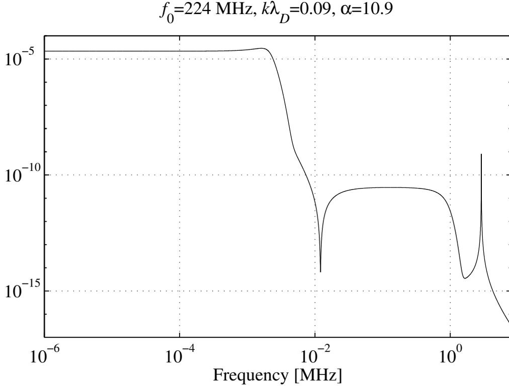
Figure 1.2: Theoretical incoherent scatter spectrum for the VHF EISCAT radar (224 MHz) for a Maxwellian plasma with  $n_e = 10^5 \text{ cm}^{-3}$ ,  $T_e = 2000 \text{ K}$ ,  $T_i = 1500 \text{ K}$ ,  $\nu_i = 10^{-2} \text{ s}^{-1}$  and  $\nu_e = 10^2 \text{ s}^{-1}$  and using the differential cross section model of Eqs. (1.7)–(1.14)
