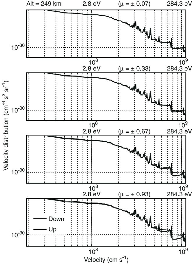
**Fig. 3.** The suprathermal angular velocity distribution function for the same eight-stream calculation at 249 km. Each plate contains two curves corresponding to two angles symmetric around the direction perpendicular to the magnetic field, i.e. the upward angular flux (*thin solid line*) and the downward one (*thick solid line*). The upper horizontal scale on each plate is energy expressed in eV
