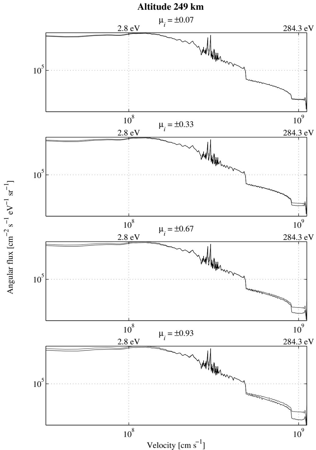
Figure 5.1: Example of the angular flux calculation for an 8-streams run over Tromsø in June 1996 at 12:00 UT with a F10.7 index of 80 and an  $A_p$  index of 15. The *thin* line is for the downward direction and the *thick* line is for the upward direction
