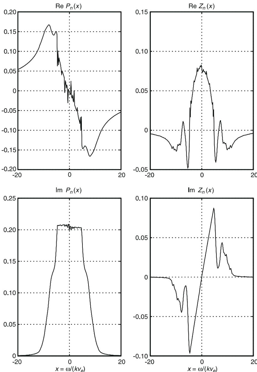
**Fig. 9.** On the left, the real and imaginary parts of  $Z_n$  for real argument and on the right, the real and imaginary parts of  $P_n$  for real argument of a suprathermal distribution at the altitude of 202 km. These calculations were performed using a 32-stream calculation of the transport code and the distribution function was then recalculated over 1024 double-Gauss points in order to perform the calculations of  $P_n$  and  $Z_n$  over this  $\mu$ -grid
