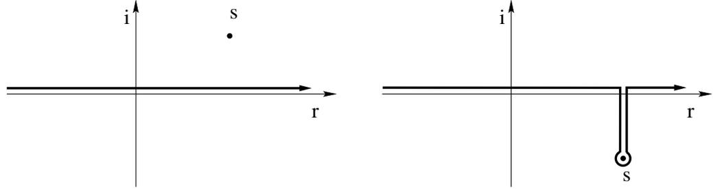
Figure 1.1: Landau contour of integration used to evaluate the integrals  $Z$  and  $P$  of Eq. (1.13) and (1.14). In the left panel,  $\nu_\alpha > 0$  while in the right panel  $\nu_\alpha < 0$
