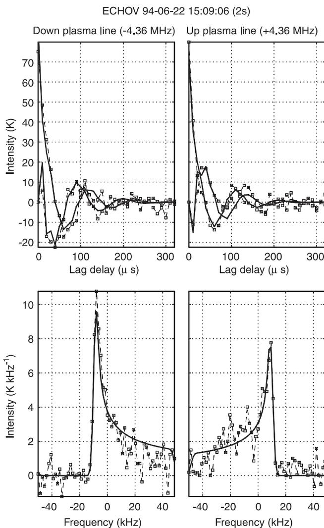
**Fig. 2.** Example of the result of a fit of the up- and downshifted plasma lines. The two *upper panels* show the measured complex autocorrelation functions expressed in units of antenna temperature (*dashed line*) and the theoretical model (*solid line*). The *curves* with the intensity equal to zero at the zero lag delay are the imaginary parts. The two *lower panels* present the corresponding power density spectrum where the critical frequency is more easily identified in the spectral shape
