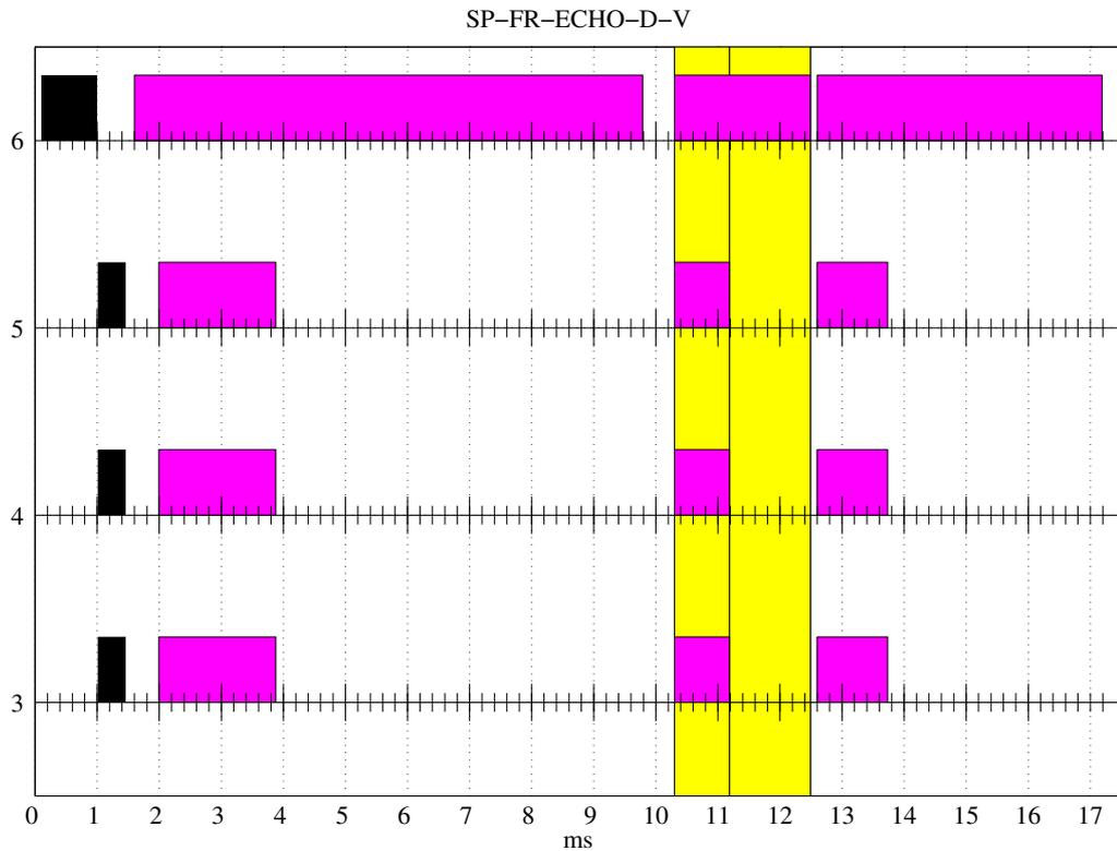
Figure 2.3: Time diagram of the pulsing of the EISCAT long pulse experiment ECHO-D-V. *black* is for the transmitted pulses, *dark gray* is for the receiving periods and *light gray* is when the calibrated noise source is injected. The background measurement is performed at the end of the cycle. The whole cycle is run in 17.5 ms and provides good statistical accuracy in a short time
