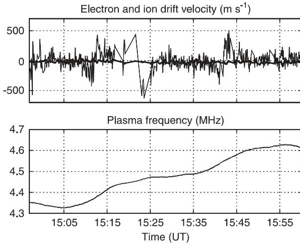
**Fig. 12.** The *upper panel* shows the estimated ion drift velocity  $u_i$  (*thick line*) from the ion line analysis and the electron drift velocity  $u_e$  (*thin line*) from the analysis method based on Eq. (8) with a suprathermal population described by the distribution function of Fig. 8 and a Spitzer function for the ambient electrons with parameters of Fig. 6. The *lower panel* shows the estimated plasma frequency  $\omega_e/2\pi$  given by Eq. (9)
