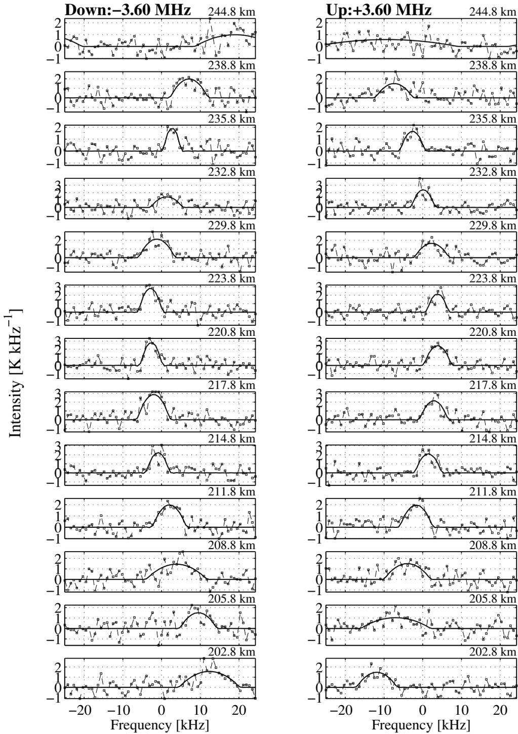
Figure 3.3: Alternating code fit of plasma line data collected with ALT32-2-V. The right panels are for the up-shifted plasma lines and the left panels are for the down-shifted plasma lines. The *dashed* lines are the estimated intensity spectra from the ACF's and the *solid* line is the fitted theoretical model
