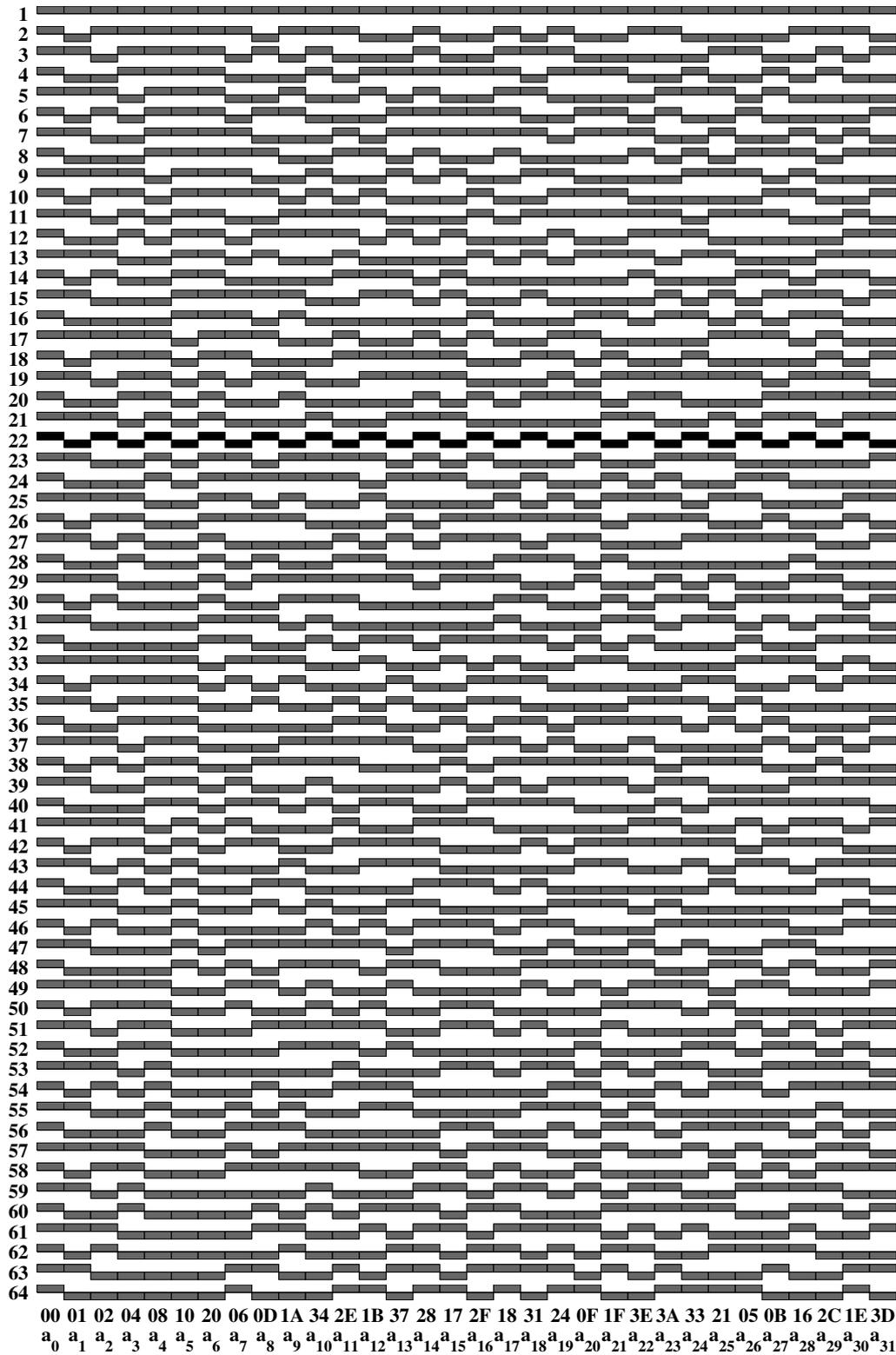
Figure 2.5: The 64 pulse sequences required for the 32 bits strong condition alternating code available at EISCAT. The  $a_i$  is the sequence of numbers needed to calculate the signs of the pulse with Eq. (2.2). The sequence  $SC = 22$  in *dark gray* is a regularly alternated modulation of period two times the length of the baud
