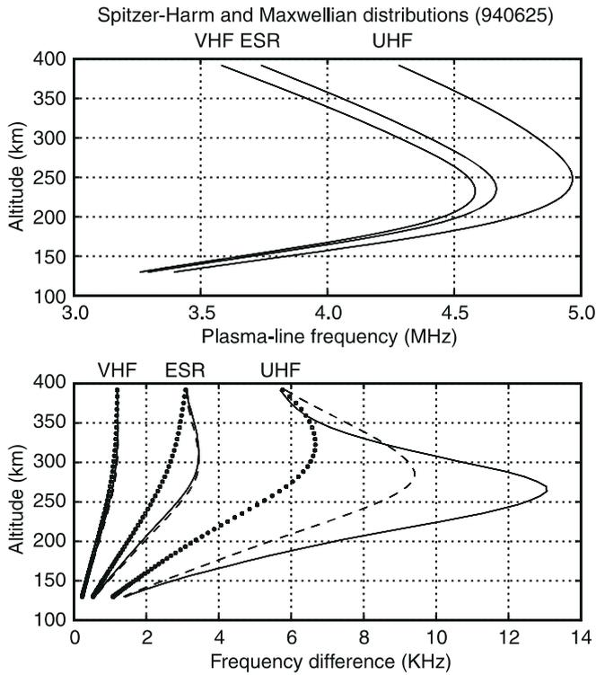
**Fig. 12.** The upper plate presents the calculated upshifted plasma frequency for the Spitzer-Härm distribution for the three different EISCAT radars. In the lower plate we present the frequency difference between up- and downshifted lines for the three radars. The Maxwellian approximation is shown with *circles*, the full two-dimensional dispersion estimation is the *solid line* and the heat flow approximation (Kofman *et al.*, 1993) is shown with the *dashed line*.
