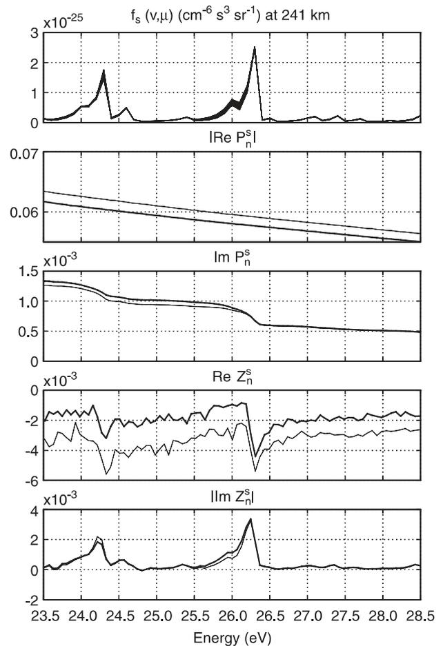
**Fig. 8.** The suprathermal electron angular velocity distribution function (*top panel*) at 241 km calculated by a 32-streams run of the transport code to gives the distribution at 32 angles and the complex functions  $P_n^s$  and  $Z_n^s$  calculated numerically with this distribution function, in the energy range 23.5–28.5 eV. The *thin line* is for downward phase energy and the *thick line* is for upward phase energy
