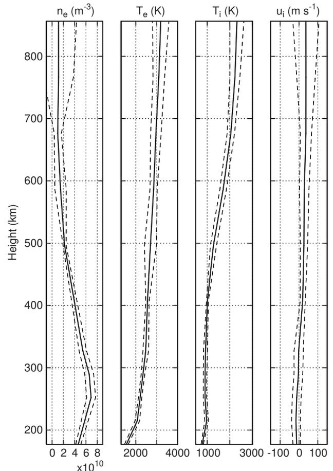
**Fig. 1.** The electron density  $n_e$ , the electron and ion line temperatures  $T_e$  and  $T_i$  and ion mean drift velocity  $u_i$  as a function of altitude averaged over the 1-h period of the experiment run. The *dashed lines* represents the  $1-\sigma$  deviation from the averaged parameter (*solid line*)
