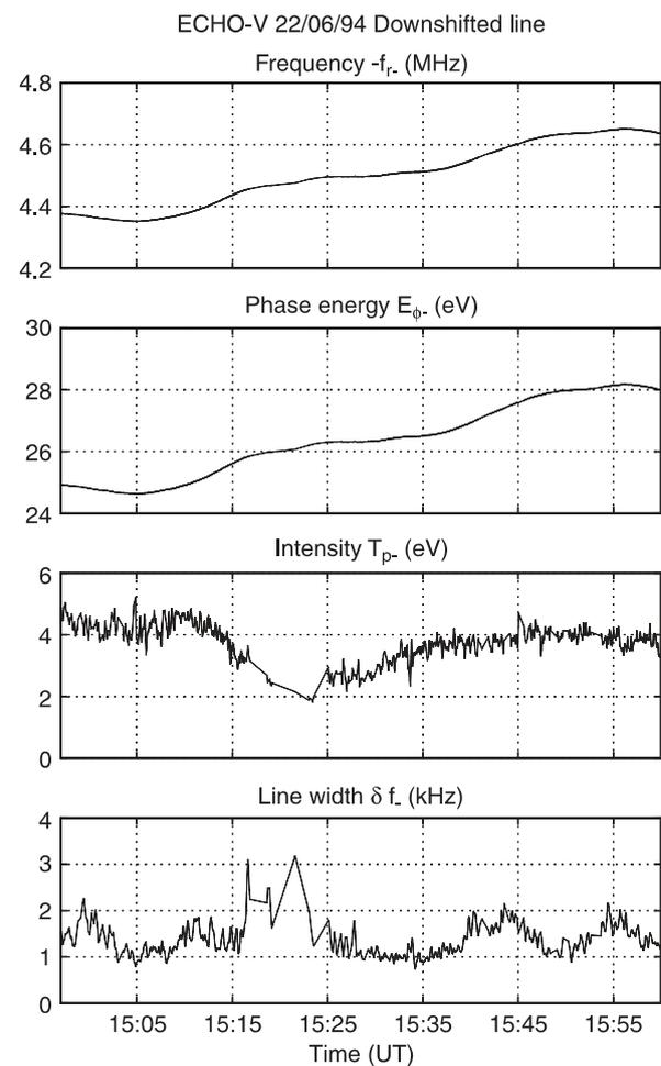
**Fig. 3.** The parameters extracted from the downshifted plasma line analysis for the 1-h period of observation. From *top to bottom*: the absolute value of the critical frequency [ $f_{r-}$ ], the corresponding phase energy  $E_{\phi-}$ , the intensity of the line (or plasma line temperature)  $T_{p-}$  and the line width  $\delta f_{-}$
