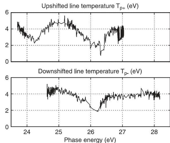
**Fig. 5.** The temperature  $T_{p+}$  and  $T_{p-}$  of the up- and downshifted plasma lines from the 1-h observation of Figs. 4 and 3 plotted as a function of their phase energy, respectively  $E_{\phi+}$  and  $E_{\phi-}$ .
