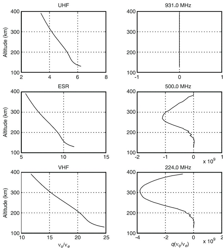
**Fig. 14.** In the left plates, the ratio  $v_\phi/v_e$  where  $v_\phi$  is the phase velocity of the Langmuir wave for the three different radars (from top to bottom UHF, ESR and VHF). In the right plates, the integrated heat flux up to the phase velocity  $v_\phi$
