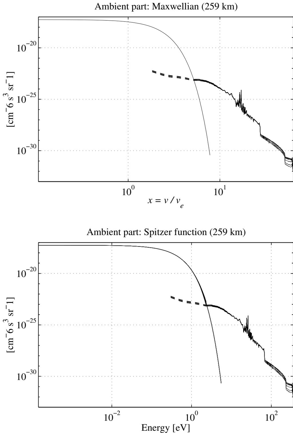
Figure 1.10: The upper plate shows both a Maxwellian and the supra-thermal distribution as a function of the dimensionless parameter  $x = v/v_e$ . The supra-thermal is truncated at the intersection with the Maxwellian. The lower plate presents the situation where the ambient distribution is the Spitzer function described in Chapter 4. The distributions are plotted as a function of the energy  $v = 1/2m_e v^2$ . The two plates are for the same altitude and same ionospheric parameters
