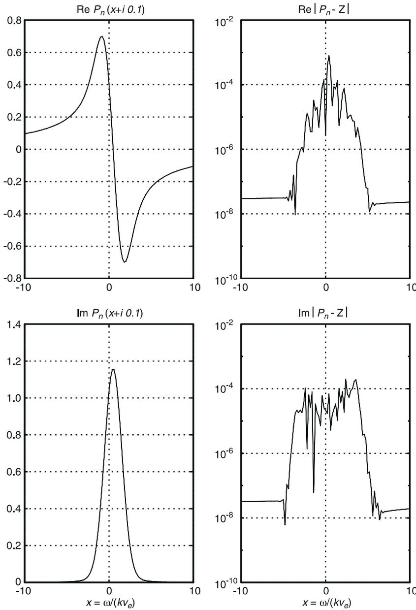
**Fig. 5.** On the left, the real and imaginary parts of the  $P_n$  function given by Eq. (35) for complex argument such that the imaginary part  $\eta = 0.1$ . On the right, their relative error with the real and imaginary parts of  $\mathbf{Z}(z/\sqrt{2})/\sqrt{2}$ , where  $\mathbf{Z}$  is the plasma dispersion function (Fried and Conte, 1961). The normalized Doppler shift of the Maxwellian distribution is  $x_d = 0.5$
