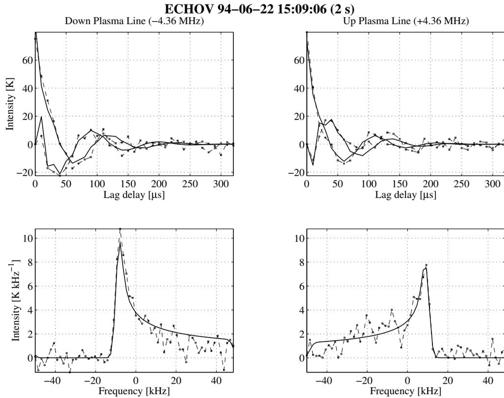
Figure 3.1: Long pulse fit of data collected with ECHO-D-V. The two upper panels show the measured complex autocorrelation functions expressed in units of antenna temperature (*dashed line* and the theoretical model (*solid line*) of Eq. (3.1). The curves with the intensity equal to zero at zero lag delay are the imaginary parts. The two lower panels present the corresponding power density spectrum where the critical frequency is more easily identified
