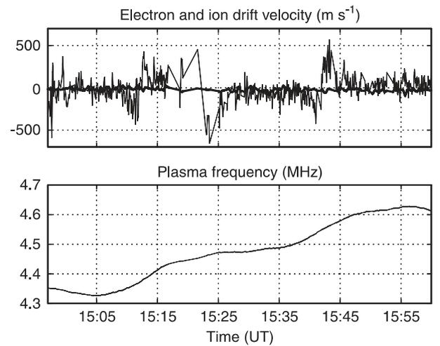
**Fig. 10.** The upper panel shows the estimated ion drift velocity  $u_i$  (thick line) from the ion line analysis and the electron drift velocity  $u_e$  (thin line) from the analysis method based on Eq. (8) without suprathermal population ( $\alpha = 0$ ) and assuming a Maxwellian ambient population with the parameters of Fig. 6. The lower panel shows the estimated plasma frequency  $\omega_e/2\pi$  given by Eq. (9)
