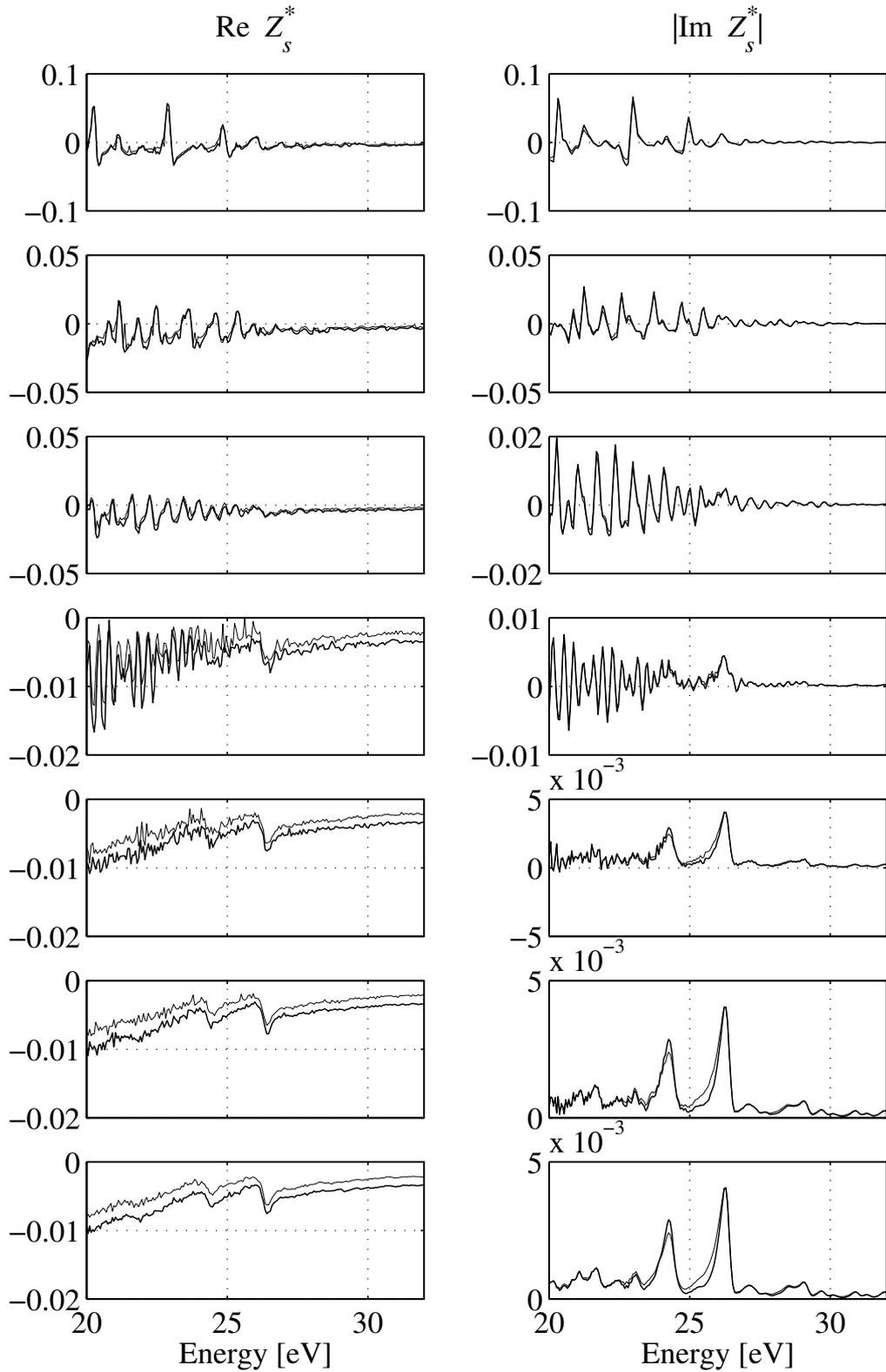
Figure 1.9: Test of the  $Z^*$  function with the supra-thermal velocity distribution calculated on a 8-streams run at 259 km (see Figure 1.7). From top to bottom the number of points in the quadrature are 32, 64, 128, 256, 512, 1024 and 2048. The *thick* line is for downward energy while the *thin* line is for upward energy
