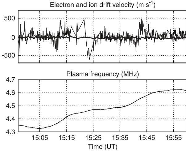
**Fig. 11.** The *upper panel* shows the estimated ion drift velocity  $u_i$  (*thick line*) from the ion line analysis and the electron drift velocity  $u_e$  (*thin line*) from the analysis method based on Eq. (8) with a suprathermal population described by the distribution function of Fig. 8 with a Maxwellian background of parameters of Fig. 6. The *lower panel* shows the estimated plasma frequency  $\omega_e/2\pi$  given by Eq. (9)
