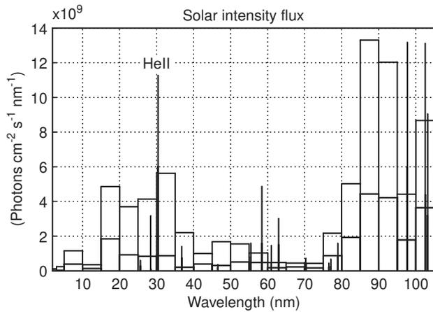
**Fig. 7.** The model for the solar intensity flux (Torr and Torr, 1985). The *thin line* is for solar maximum ( $F_{10.7} = 243$ ) and the *thick line* for solar minimum ( $F_{10.7} = 68$ ). The solar flux for any arbitrary  $F_{10.7}$  is deduced by interpolation between these two references fluxes
