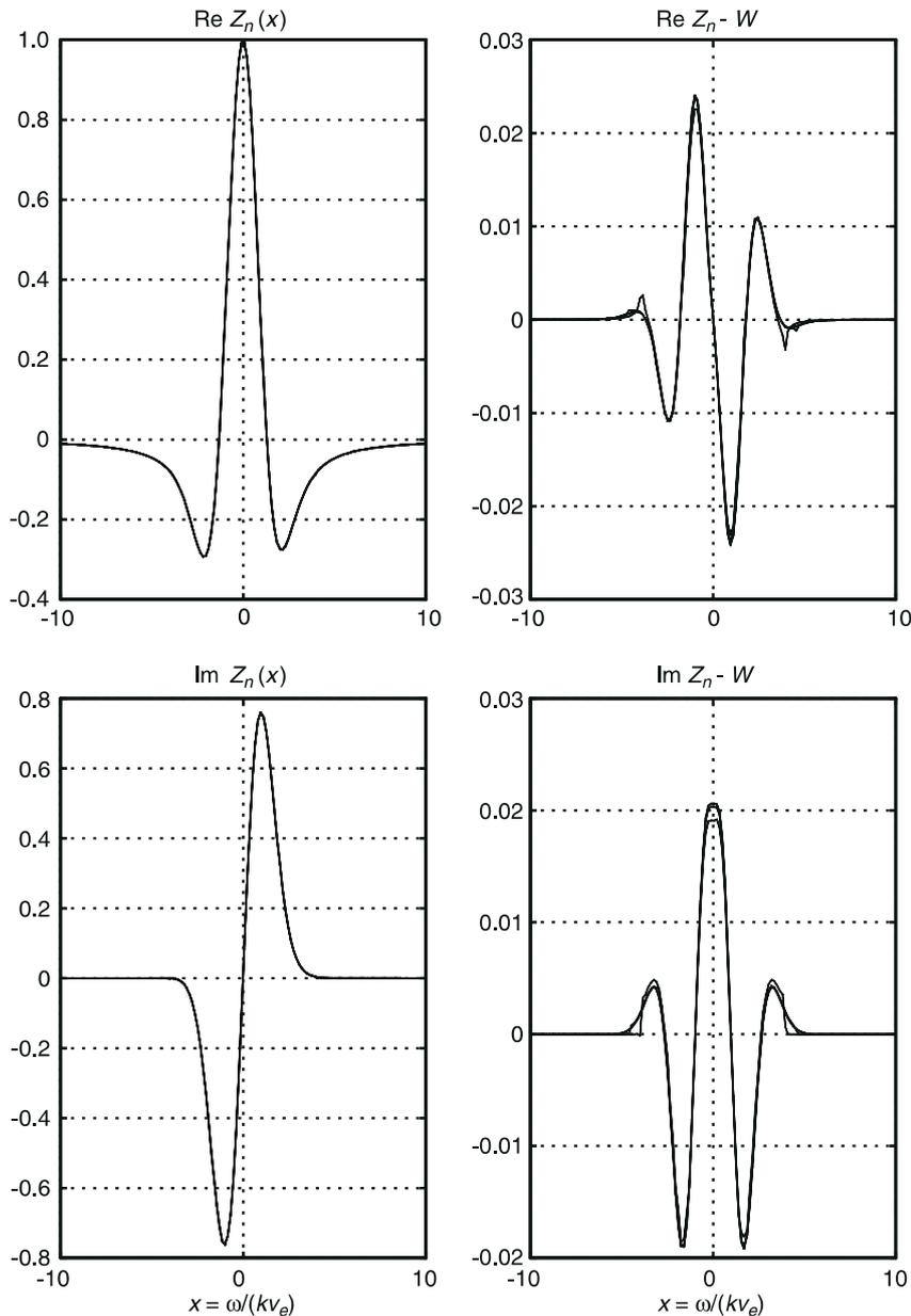
**Fig. 8.** On the left, the real and imaginary parts of  $Z_n$  for real argument and for  $\epsilon_T = 5 \cdot 10^{-2}$  and  $\epsilon_E = -3\epsilon_T\gamma_T/4\gamma_E$ . On the right the difference between  $Z_n$  and  $W$  for the four different values of  $x_{\max}$  of Table 1
