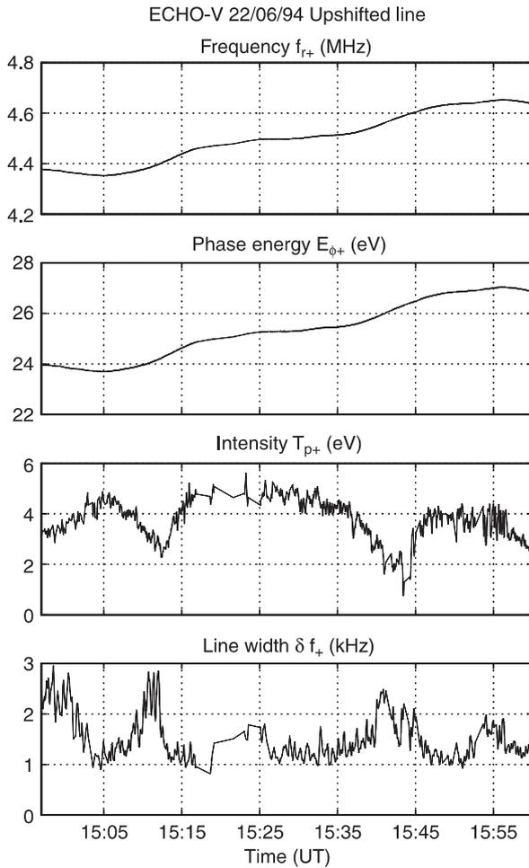
**Fig. 4.** The parameters extracted from the upshifted plasma line analysis for the 1-h period of observation. From *top to bottom*: the critical frequency  $f_{r+}$ , the corresponding phase energy  $E_{\phi+}$ , the intensity of the line (or plasma line temperature)  $T_{p+}$  and the line width  $\delta f_+$ .
