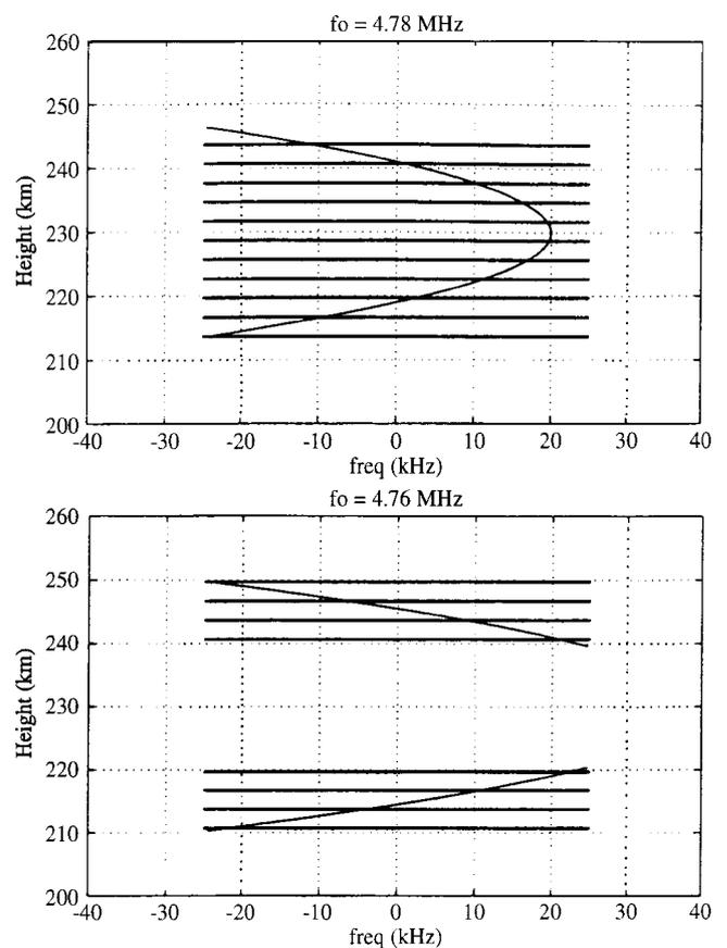
**Fig. 1.** Parabolic height distribution of the plasma-line frequency with scale height of 65 km showing two different tunings of the 50-kHz receiving filter and the corresponding height cells contributing to the scattering
