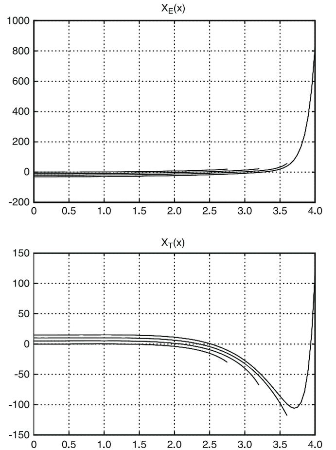
**Fig. 1.** The perturbation functions  $X_E$  and  $X_T$  integrated to different upper boundary  $x_{\max} = v/\sqrt{2}v_e = 2.8, 3.2, 3.6$  and  $4.0$ , and for an ion charge number  $Z=1$ . Note that  $X_E(0)=X_T(0)=0$  and that the  $X_E$ 's are shifted by  $-10$  with each other, the  $X_T$ 's are shifted by  $+5$  with each other, the reference curves (i.e. not shifted) are for  $x_{\max} = 2.8$
