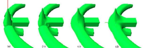
**Fig. 4** Blending operations: (a) Initial object composed as a vertical cone, a torus-like shape and a block shape. (b) Blending between the block and the cone. (c) Blending between the torus and the cone. (d) Blending between the block and the cone, and blending between the previous resulting object with the torus.
