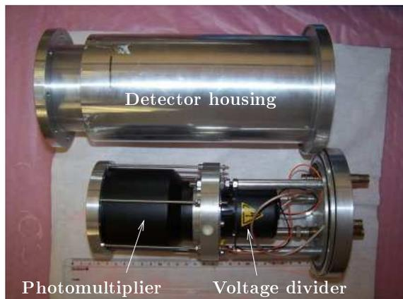
**Figure 10.2:** Set-up of the scintillator detectors.
