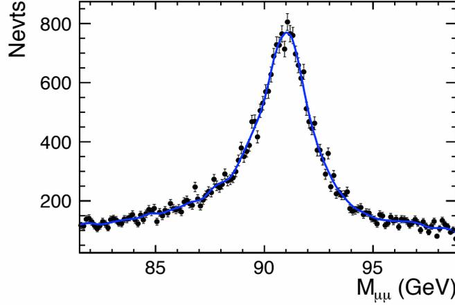
Figure 6.34: Fit of the *Invariant Mass* of the  $Z \rightarrow \mu^+ \mu^-$  in the ZZ process using *Kernel Estimation*, with polarization mode  $e_L^- e_R^+$ . An accuracy of 13 MeV is obtained for the invariant mass measurement.
