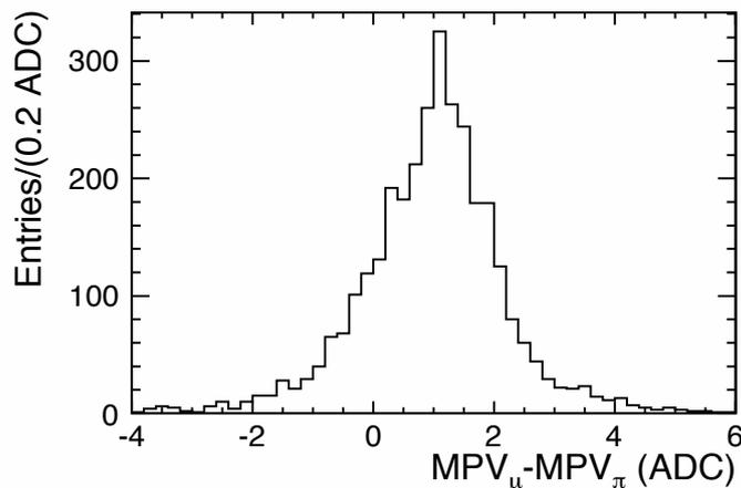
Figure 5.11: Differences of the calibration constants for each pad, between that obtained from muons with  $20 \times 20$  trigger and from pions with  $10 \times 10$  Čerenkov, with a mean of  $0.97 \pm 0.02$  ADC counts and a RMS of  $1.19 \pm 0.02$  ADC counts.
