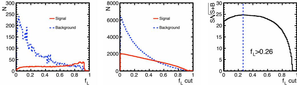
Figure 6.17: The distributions of the Likelihood Fraction  $f_L$  (left), the number of remaining events versus the cut on  $f_L$  (middle), and the significance versus  $f_L$  cuts (right). The distributions are shown for the  $\mu\mu X$ -channel with polarization mode  $e_L^- e_R^+$  in the MI Analysis.
