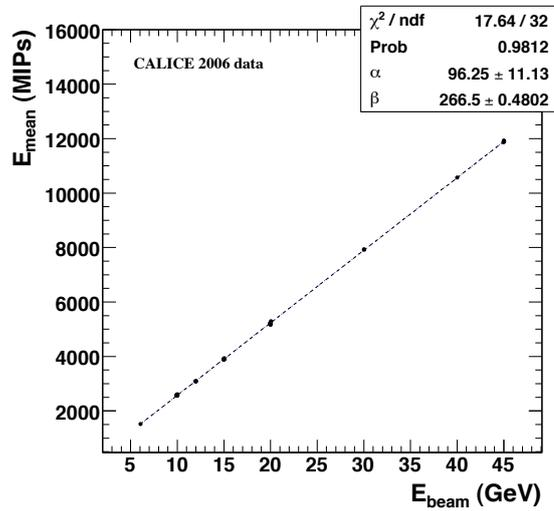
Figure 4.5: Energy responses of the prototype as a function of the beam energy[33].
