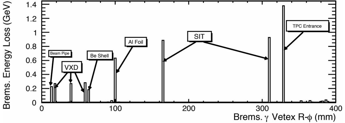
Figure 3.11: Mean Bremsstrahlung energy loss as a function of the Bremsstrahlung photon vertex in the barrel region of the ILD detector, for electrons in the Higgsstrahlung sample with  $Z \rightarrow e^+e^-$ . The vertices correspond to the positions of the detector components as labeled, with the mean energy loss proportional to the amount of material.
