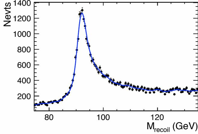
Figure 6.35: Fit of the *Recoil Mass* to the  $Z \rightarrow \mu^+\mu^-$  in the  $ZZ$  process using *Kernel Estimation*, with polarization mode  $e_L^-e_R^+$ . An accuracy of 28 MeV is obtained for the  $Z$  recoil mass measurement.
