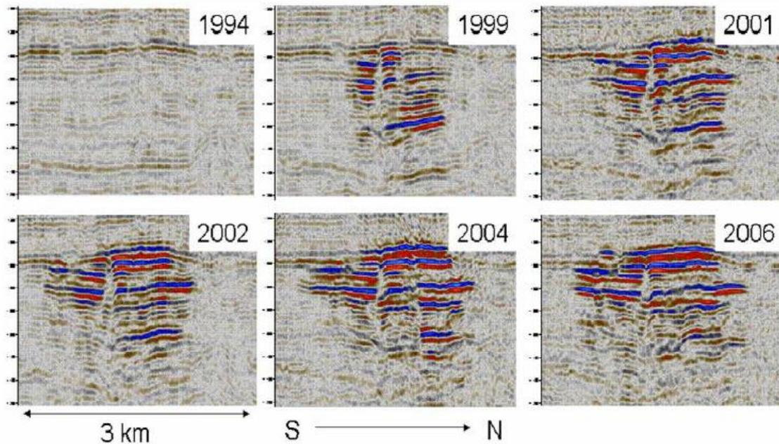
Figure 1.2 Time lapse seismic data in the Utsira Formation. The bright amplitudes reveal the presence of injected CO<sub>2</sub>. (From Hermanrud et al., 2009)
