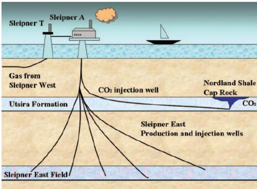
Figure 1.1 Cross section of CO<sub>2</sub> injection in the Utsira formation at Sleipner (from Audigane et al, 2007)
