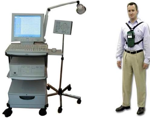
Figure 2.6: EEG recording systems. Left: Stationary system. Right: Ambulatory system (Grass Telefactor)
