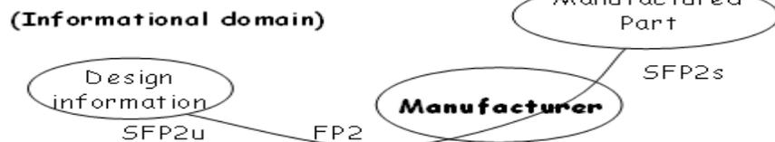
SFP2u: solid material or/and atom (electron) + information amount + ... - **FP2: Convert** - SFP2s: solid material + volume + dimensions + shape+...
