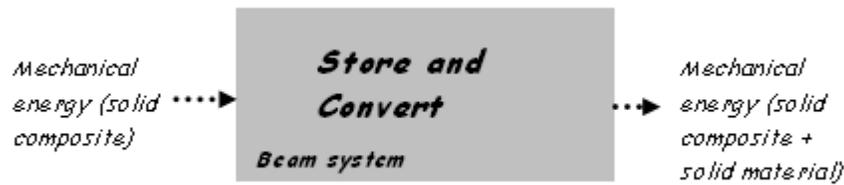
Figure 93: Functional structure of a beam
