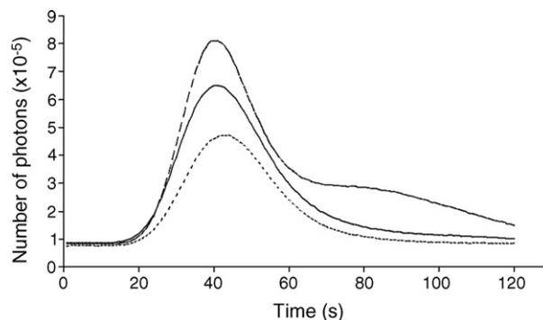
Fig. 3. Chemiluminescence peaks obtained by injection of seawater + 6 nM of hemin in different carriers: MQ water (dotted line), NaCl (0.5 M) (dark gray line) and artificial seawater (light gray line).
