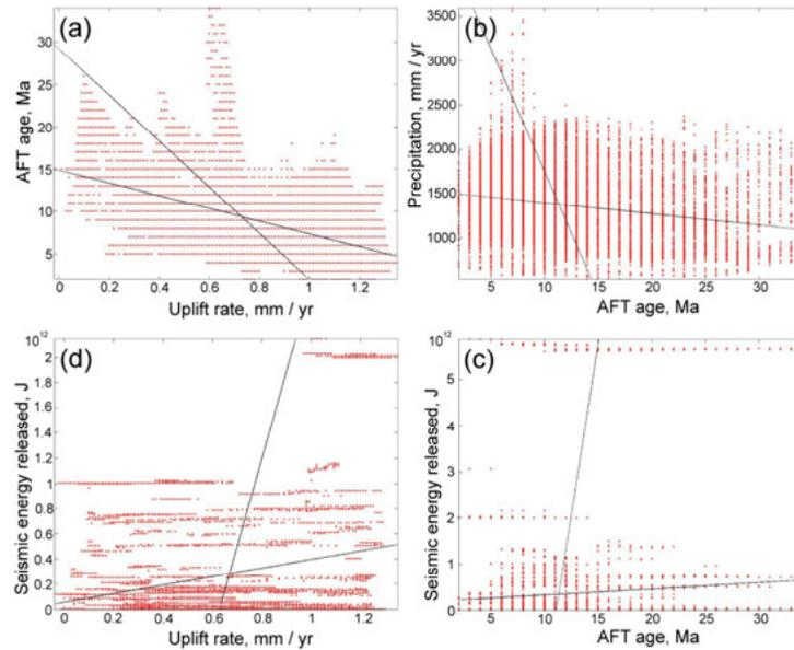
Figure III.1. Examples of 4 plots used in the search for correlation in the parameters space: (a) example of a “strong” correlation (AFT age vs. uplift rate), (b) “weak” correlation (AFT age vs. precipitation), and (c, d) no correlation (Uplift rate and AFT age vs. seismic energy released).
