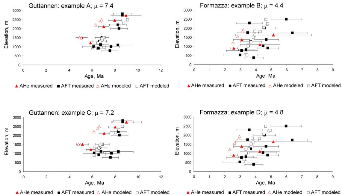
Figure IV.2.14. Comparison between measured AHe and AFT ages, and predicted ages using *Pecube* modeling.  $\mu$  is the value of cumulated misfit used to quantify the gap between measured and predicted ages (see equation IV.2.1). Examples A and C correspond to the two best models in Guttannen, (see Figures IV.2.10 and IV.2.12), and examples B and C to the best models in Formazza (see Figures IV.2.10 and IV.2.13).
