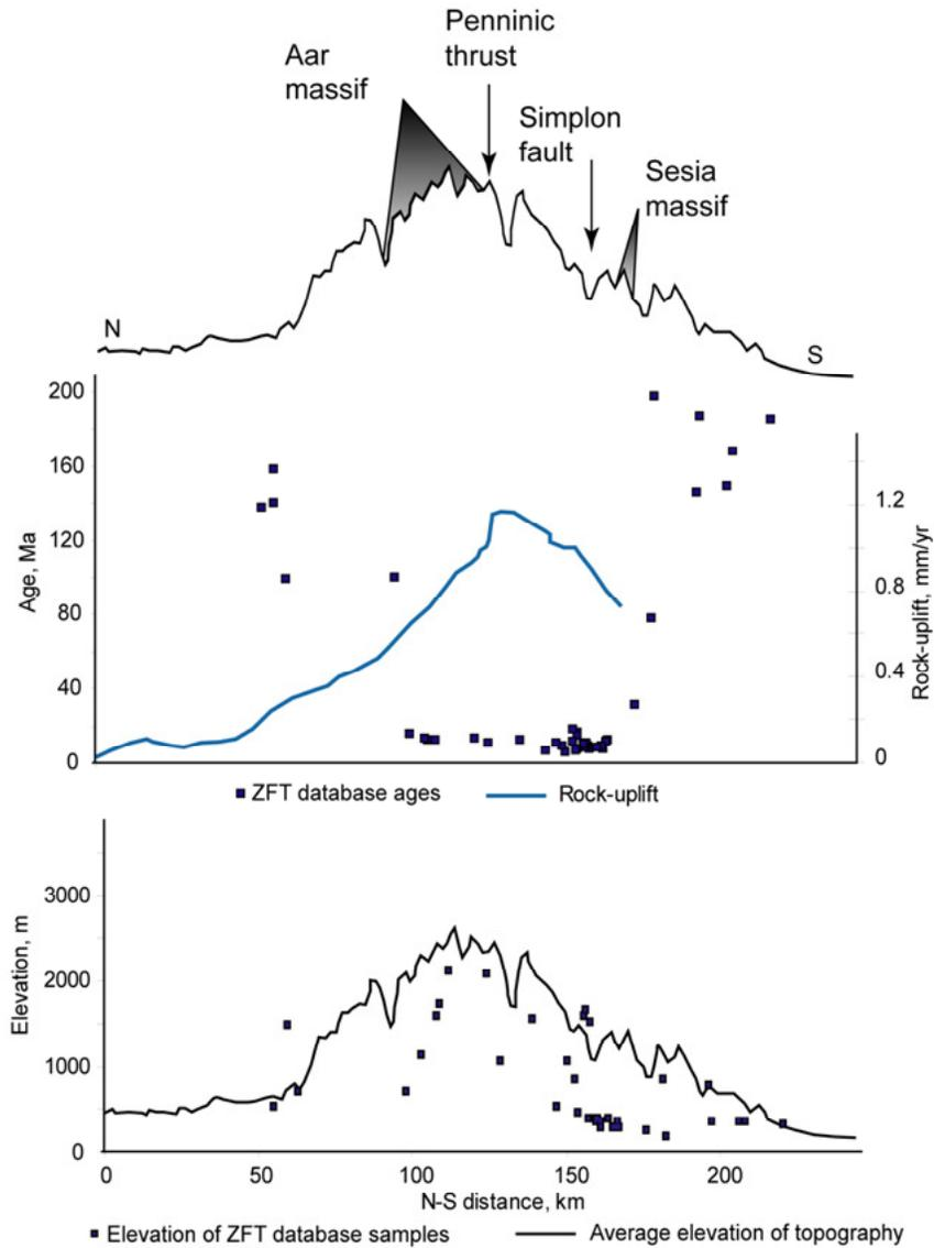
Figure III.3.5. ZFT ages across the Aar-Lepontine section. "ZFT database ages" are described in section II.2, and "rock uplift" in section III.2. The lower panel presents the elevation of samples dated, superposed on the average topography.
