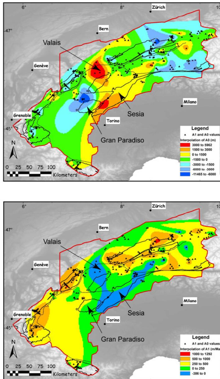
Figure II.3.6. Interpolation of the A1 and A0 values calculated to define the optimum age-elevation relationship in the neighbourhood of each datapoint, such as  $z = A1 \times t + A0$ , where  $z$  is the elevation in m above sea level,  $t$  the AFT age in Ma, A1 the slope of the age-elevation relationship, and A0 the ordinate at origin, i.e. the projected elevation for zero age according to the AFT ages at outcrop. See Figure II.2.3-a for references to original data.
