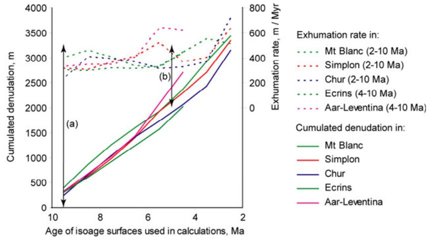
Figure II.3.33. Exhumation rate and cumulated denudation. The exhumation rates in five study areas (dotted coloured lines) estimated between 10 and 2 Ma using isoage surfaces (see locations on the lower Figure II.3.8 and original data in Figure II.2.10) allow us to estimate cumulated denudation (plain coloured lines) through time.
