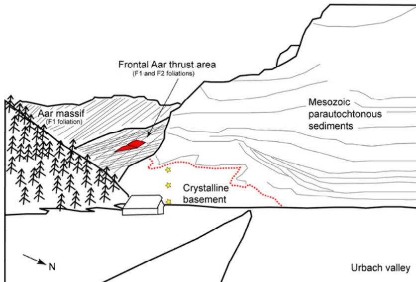
Figure IV.3.14. North verging thrust (see red arrow) at the northern Aar massif boundary, in the Urbach valley (location on Figures IV.3.11 and IV.3.15). The thrust, parallel to the F2 foliation, passes over the crystalline basement covered by Mesozoic sediments (red dotted line shows the discordance). The three yellow stars show the location of three AFT samples separated by approximately 100 m in elevation.
