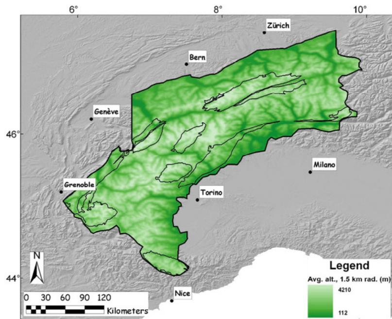
Figure III.2.11. Mean elevation in a 1.4 km radius, calculated using the DEM obtained from the CGIAR-CSI SRTM 3-arc second resolution database (<http://srtm.cs.cgiar.org>).
