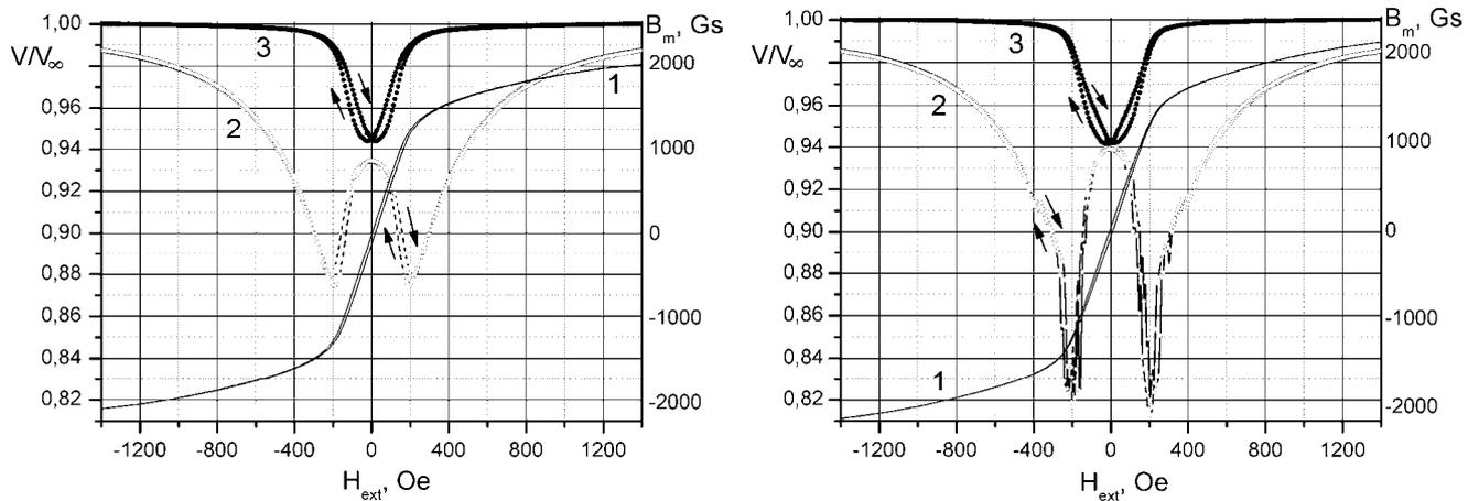
**Fig. 2. Dependencies of normalized transversal sound velocity on external magnetic field for (a) sample №4 and (b) sample №1. Curve (2) corresponds to geometry  $\vec{k} \parallel \vec{H}$  (see Fig. 1. b), curve (3) corresponds to geometry  $\vec{k} \perp \vec{H}$  (see Fig. 1. c). (1) is the hysteresis loop for corresponding samples,  $B_m = B(H_{ext}) - H_{ext}$   $H_{ext}$  is the external magnetic field.**
