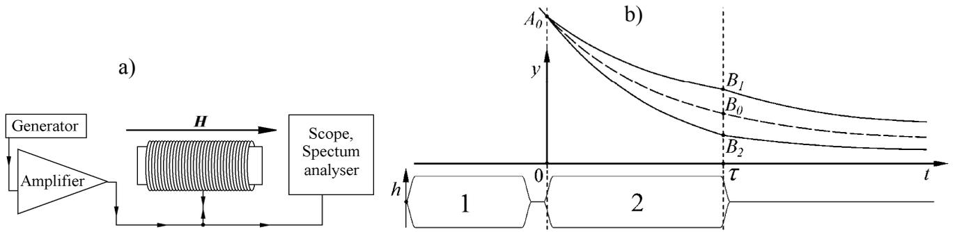
**Fig. 9.** (a) Scheme of the experiment, (b) time-diagram of the experiment: 1 – exciting pulse at resonance frequency, 2 – pulse of parametric pumping at double frequency,  $h$  – amplitude of pulses,  $y$  – amplitude of oscillations,  $A_0$  – oscillation amplitude after first pulse,  $B_0$  – free decay amplitude at moment  $\tau$ ,  $B_{1,2}$  – decay amplitude at moment  $\tau$  under parametric pumping,  $\tau$  – duration of the parametric pumping pulse.
