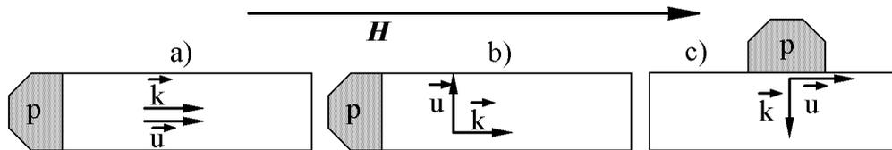
**Fig. 1. Scheme of experiment. Possible geometries of experiment: (a) longitudinal wave, (b, c) transversal wave,  $p$  is piezotransducer,  $\vec{k}$  is the wave vector,  $\vec{u}$  is the displacement vector.**
