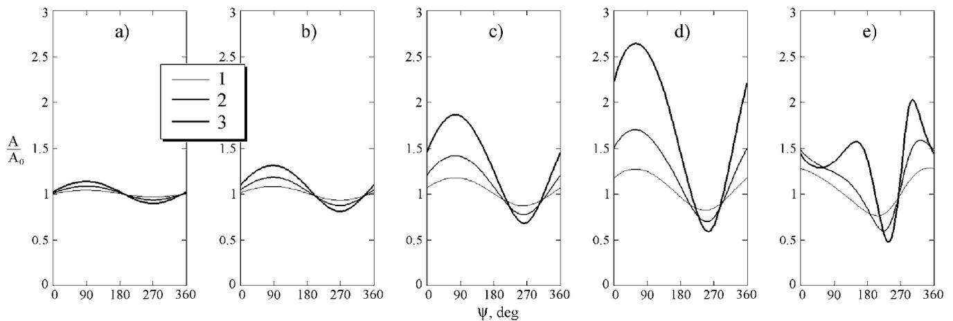
**Fig. 13.** Calculated dependences of the relative amplitude of magnetoelastic oscillations on the phase of pumping for the conditions identical with those of Fig. 12.
