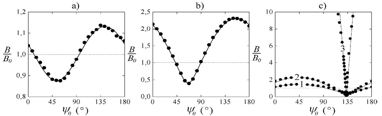
**Fig. 10.** Experimental (points) and calculated (curves) relative amplitudes of oscillations in the Terfenol-D based composite (a), the porous ferrite (b), and control ferrite (c) vs. phase shift between exciting and pumping pulses. Pumping field amplitude: the composite:  $h = 253$  Oe, the porous ferrite:  $h = 35$  Oe, and the control ferrite: 1.5 Oe (1), 2.9 Oe (2), 15 Oe (3).
