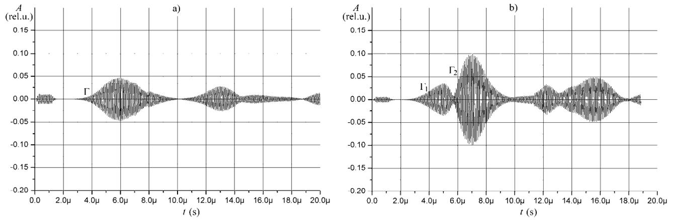
**Fig. 6. Signal waveform of conjugated waves obtained with samples (a) №4 and (b) №1. Corresponding values of amplification increment:  $\Gamma = 2.03 \mu\text{s}^{-1}$ ,  $\Gamma_1 = 2.4 \mu\text{s}^{-1}$ ,  $\Gamma_2 = 4.47 \mu\text{s}^{-1}$ .**
