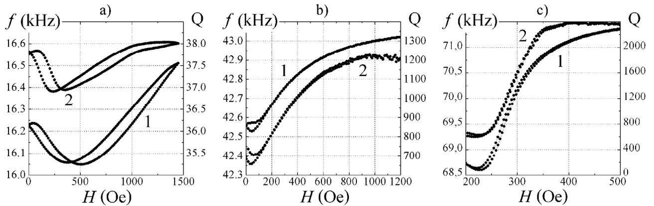
**Fig. 8.** Dependencies of the fundamental mode frequency (1) and Q-factor (2) on the DC magnetic field for the (a) composite, (b) porous ferrite, and (c) control ferrite samples.
