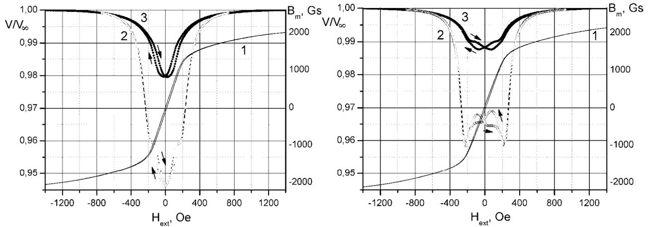
**Fig. 5. Dependencies of normalized longitudinal sound velocity correspond to geometry  $\vec{k} \parallel \vec{H}$  (3) and resonants mode frequency (2) on external magnetic field for (a) sample №4 and (b) sample №1. (1) is the hysteresis loop for corresponding samples,  $B_m = B(H_{ext}) - H_{ext}$  is the external magnetic field.**
