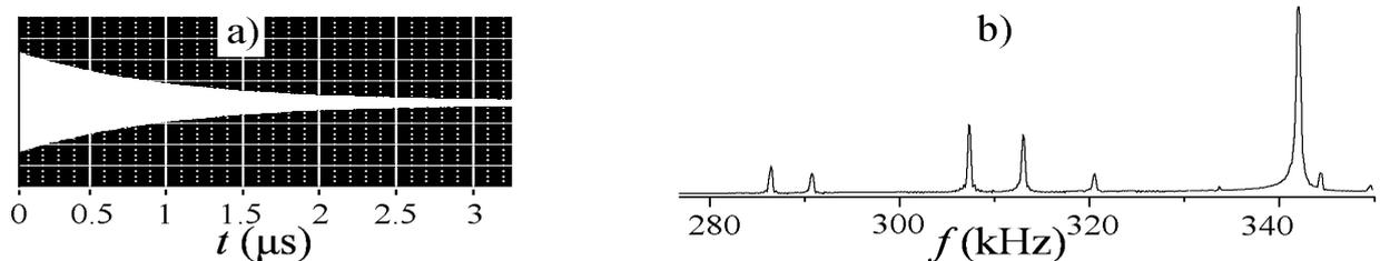
**Fig. 7. (a) Free decay oscillation of magnetoelastic mode of a ferrite sample. (b) Spectrum of resonant modes of the same sample.**
