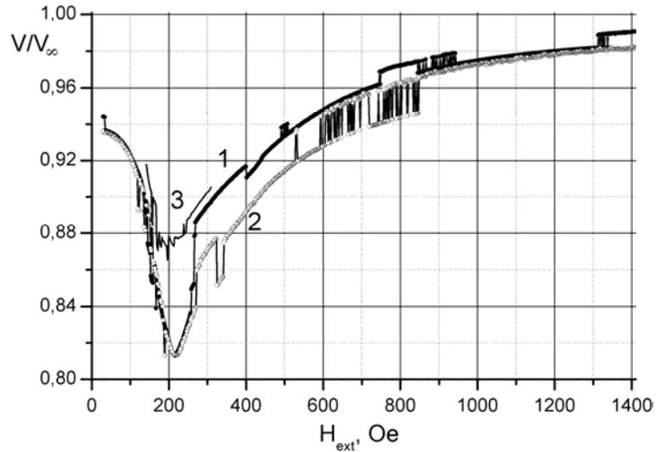
**Fig. 4.** Dependency of normalized transversal sound velocity on external magnetic field for sample №1, geometry  $\vec{k} \parallel \vec{H}$  (see Fig. 1.b). Curve (1) corresponds to 5 MHz sound, curve (2) corresponds to 1.4 MHz sound, curve (3) corresponds to 5 MHz sound with decreased sensitivity level which allows watching first of the divided pulses (see Fig. 4, d).
