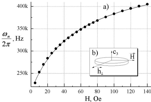
**Fig. 11. (a) Frequency of the quasi-phonon mode versus the strength of the bias magnetic field. (b) Geometry of the experiment.**
