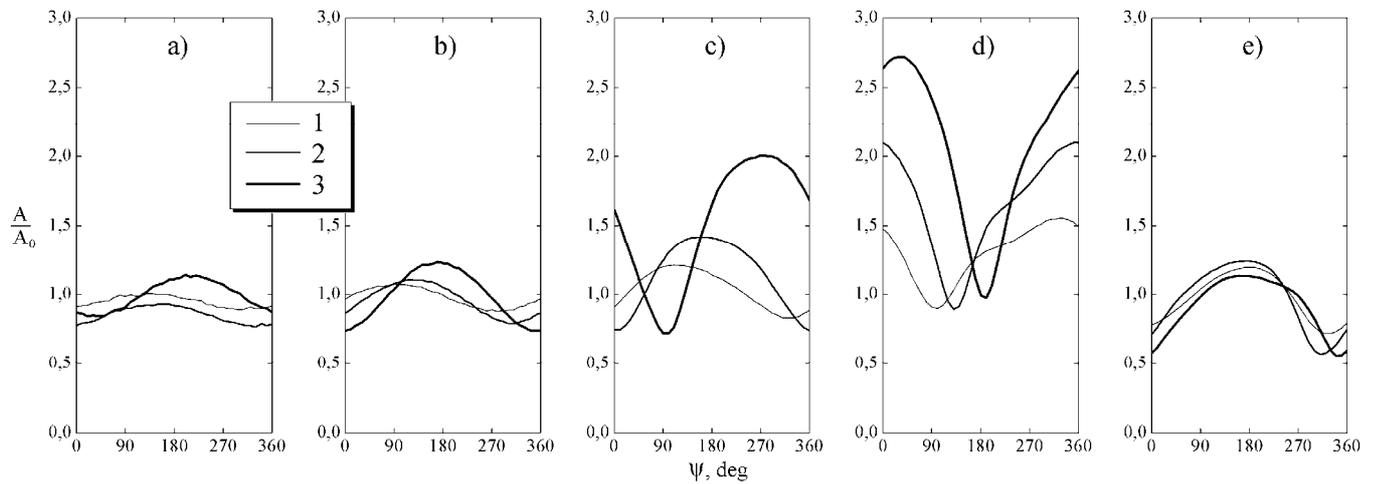
**Fig. 12.** Experimental dependences of the relative amplitude of magnetoelastic oscillations on the phase of pumping. The strength of the excitation field at the frequency  $\omega_n$  is: (a) 65, (b) 127, (c) 256, (d) 387, and (e) 635 mOe. The strength of the pumping field at the frequency  $3\omega_n$  is: (1) 0.5, (2) 0.86, and (3) 1.57 Oe.
