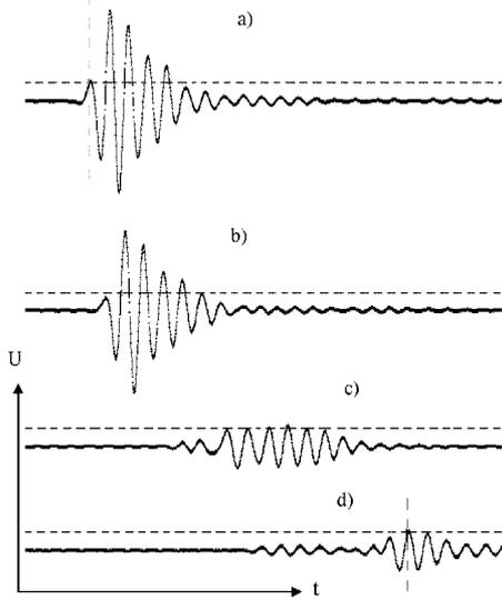
**Fig. 3.** Oscillograms of registered ultrasonic pulse for sample №1 with different values of external magnetic field: (a)  $H=660$  Oe; (b)  $H=600$  Oe; (c)  $H=400$  Oe; (d)  $H=270$  Oe. Horizontal dotted line is the sensitivity threshold, vertical dotted line is the defined delay duration.
