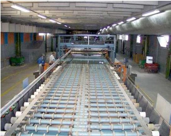
Figure 4.12: The glass ribbon is then cut into glass sheets
