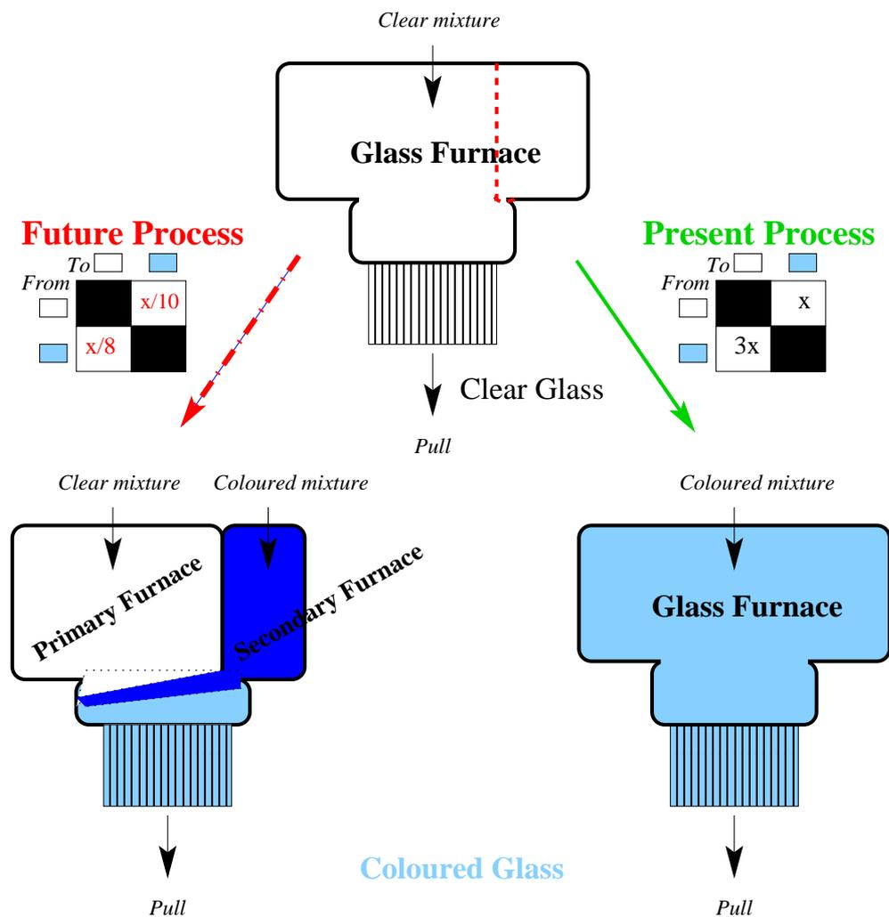
Figure 6.29: Illustration of a possible revolution in the coloration process
