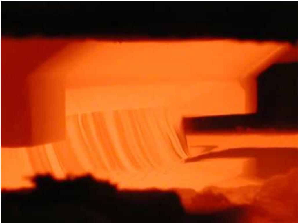
Figure 4.6: Under the spout lip: the glass flows from the furnace to the tin bath
