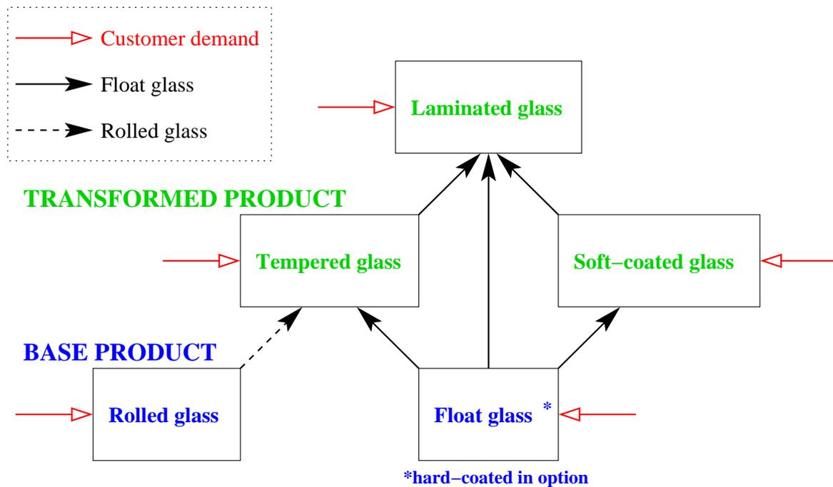
Figure 1.1: Steps of production and transformation of flat glass
