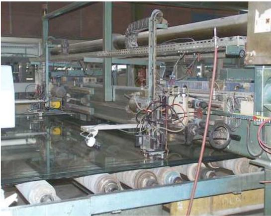
Figure 4.11: The glass ribbon is then cut to its net width
