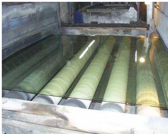
Figure 4.10: The glass ribbon inside the annealing zone
