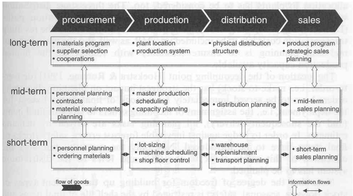
Figure 1.12: Planning tasks according to the SCP-matrix (cf. [FMW02], Fig 4.3)
