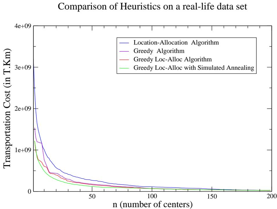
Figure 3.13: Comparison of four Heuristics of clustering on a real-life data set (200 customers)
