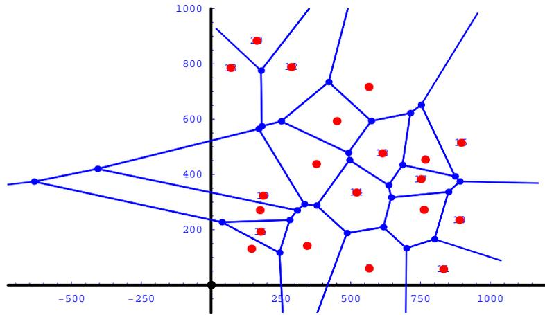
Figure 3.3: Example of Voronoi diagram on a set of 20 points
