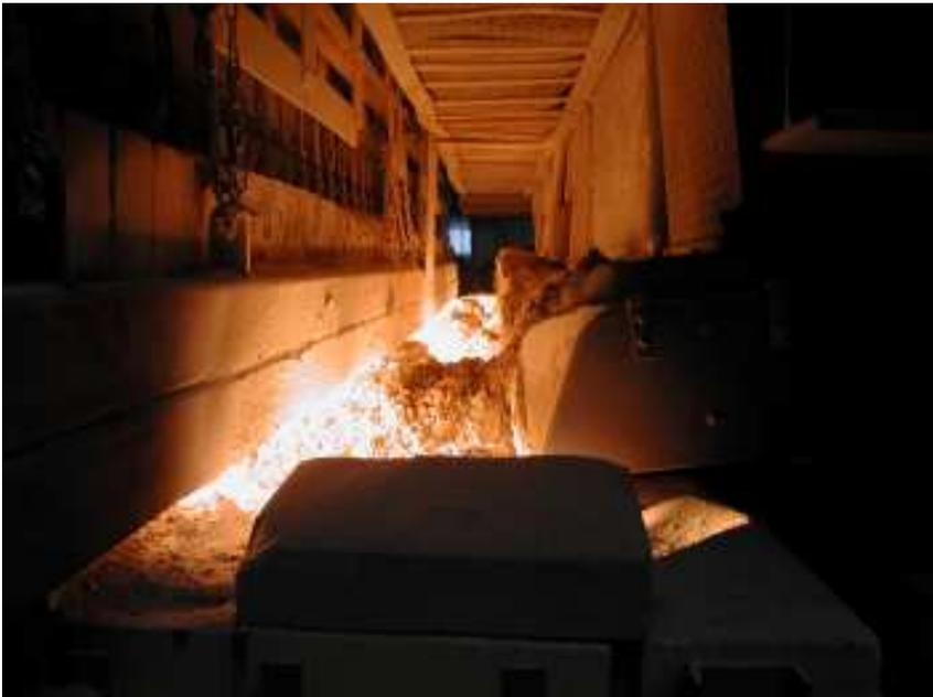
Figure 4.3: Raw materials entering the furnace
