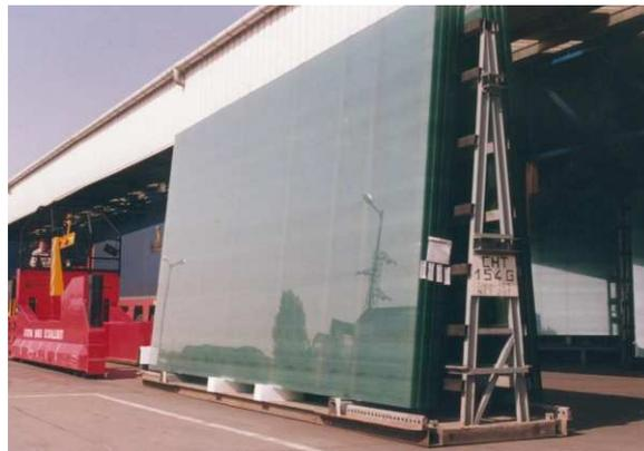
Figure 1.2: Trestle of glass ready to be loaded by an inloader
