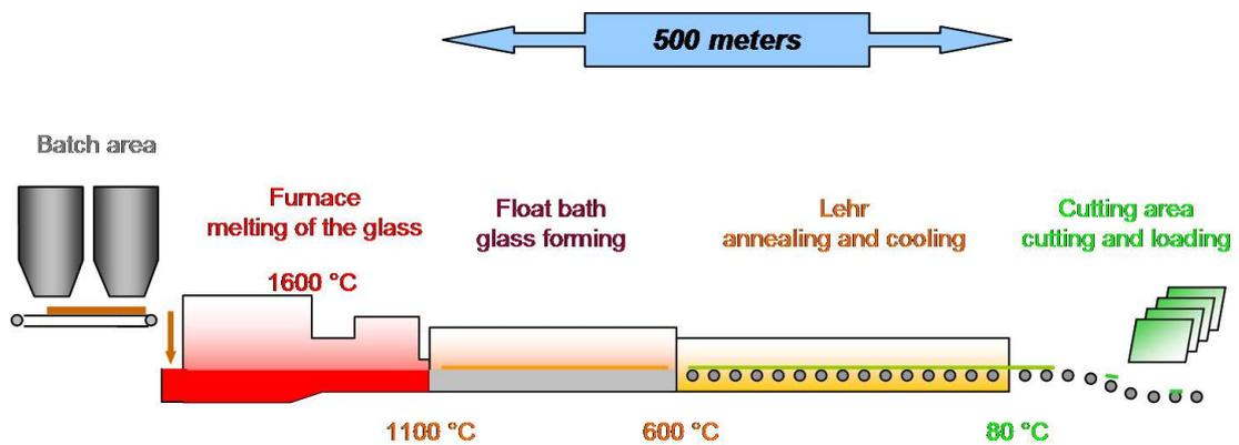
Figure 4.1: Global View of the float glass process
