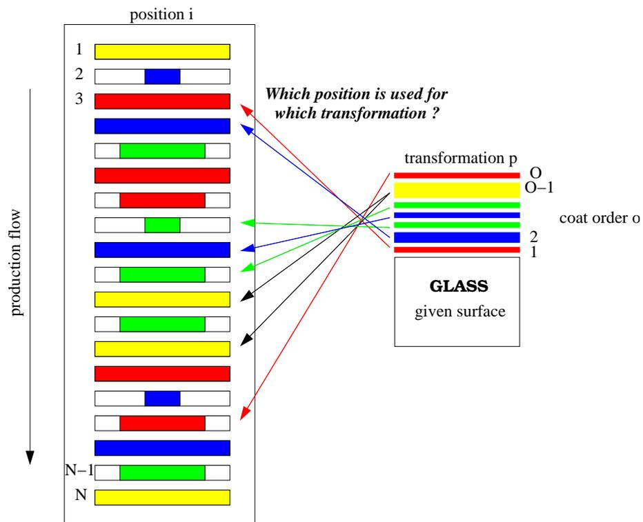
Figure 5.2: Impact of the design on the sputtering process
