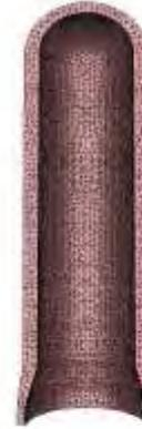
Figure 12 : Mesh of the preform (44 403 nodes, 223 155 elements).
