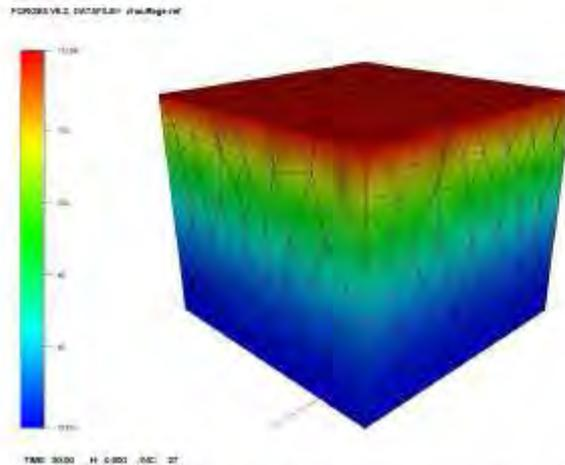
Figure 5 : Mesh used for the temperature calculation (°C).
