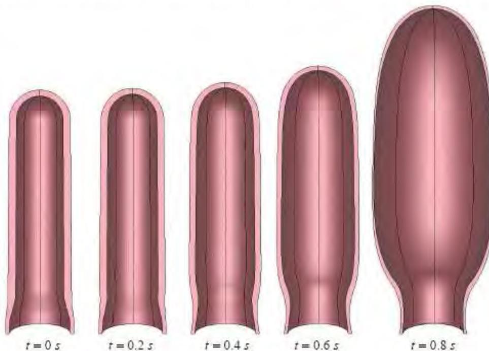
Figure 13 : Intermediate preform free inflation (CPU time = 6 hours).
