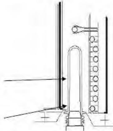
Figure 3 : Infrared heating of the preform.
