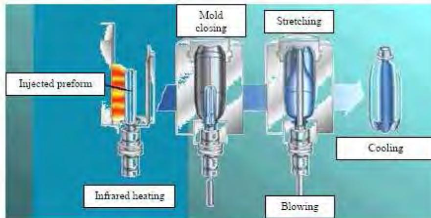
Figure 1 : Scheme of the injection blow molding process.
