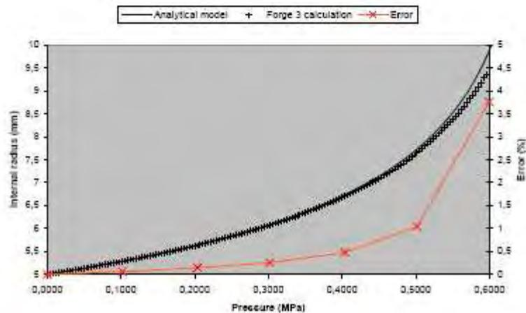
Figure 11 : Internal radius variation versus pressure.
