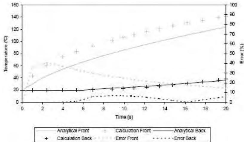
Figure 6 : Evolution of temperature in polyethylene sheet.
