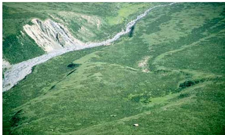
Figure 5.1 – *Lateral offset of terraces along the Haiyuan fault (China).*
