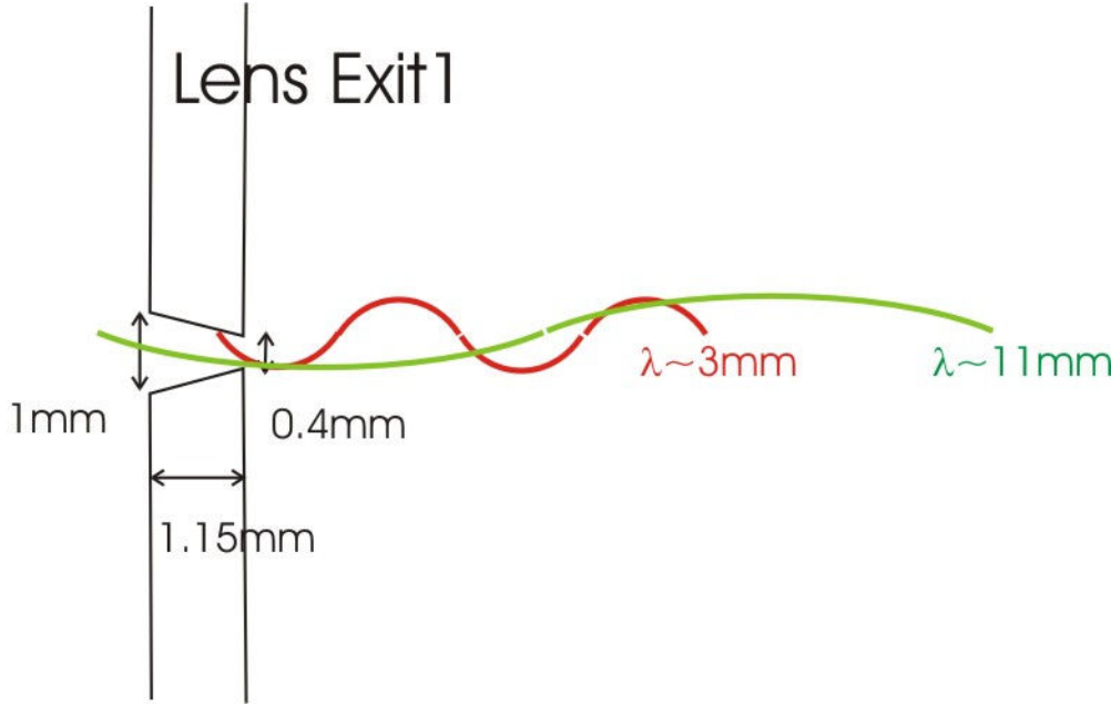
Figure 1-6 : Passage through the exit aperture in dependence with the forward velocity of electrons. Both trajectories have the same gyroradius (corresponding to transverse kinetic energy of 2K \sim 0.2\text{eV} ) but different forward velocity, the electron with the fastest forward speed can pass the aperture, the other is rejected.
