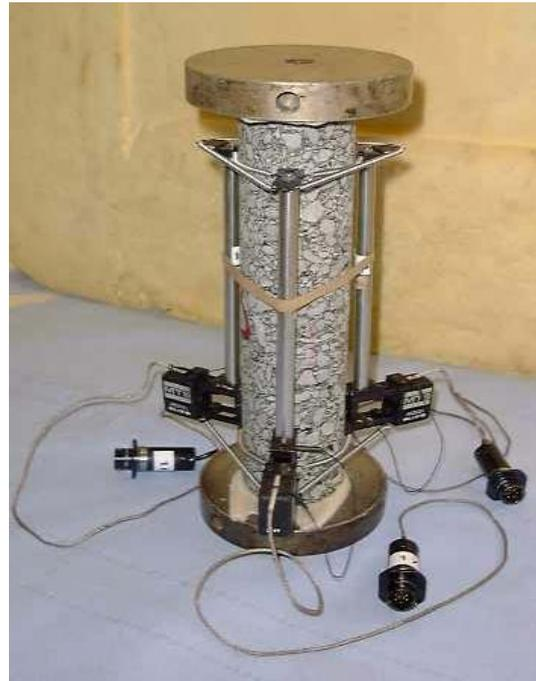
Figure III-12. Eprouvette type TSRST.
