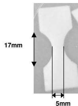
*II.3.5.2. Tensile test on regenerated cellulose + reinforcing fibres*
