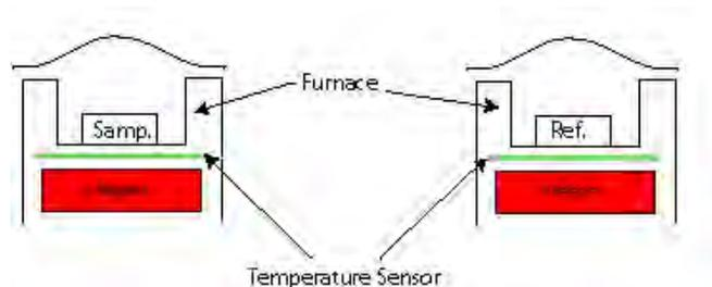
Fig.II.3-1: Diagram of a power-compensated DSC
