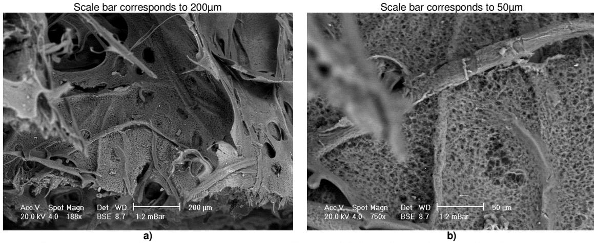
**Sponges made from the viscose process: cellulose Rayonier DP1044 with a mixture of cotton, flax and fluff regeneration in water at +70 $^{\circ}$ C**
