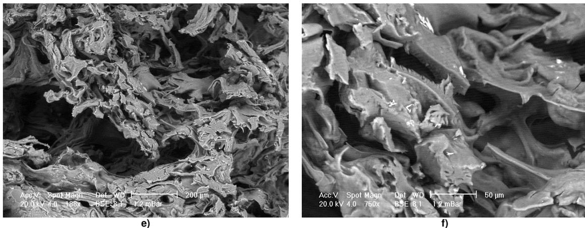
**Sponges made from the NaOH process: 5B389 cellulose/7.6NaOH/water with 2 reinforcing fluff fibres pre-impregnated with 8%NaOH/water at -6 $^{\circ}$ C, porophores added, 20 hours of gelation at +25 $^{\circ}$ C, regeneration in water at +70 $^{\circ}$ C.**
