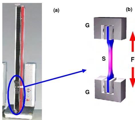
Fig.II.3-9: Picture of the Zwick Z2.5 machine and scheme of the tensile test.
