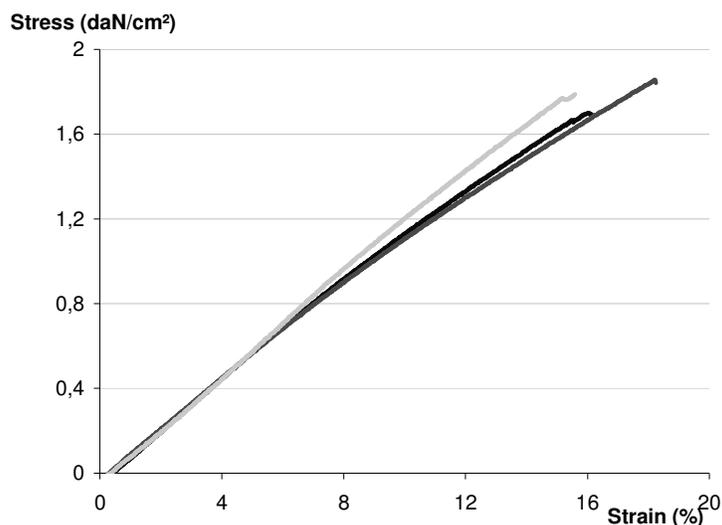
**Fig.2-1: Example of a tensile test on a regenerated cellulose solution initially containing 5B407 cellulose/7.6NaOH/water; solution was frozen for 20 hours at -20°C and regeneration in water at +70°C.**
