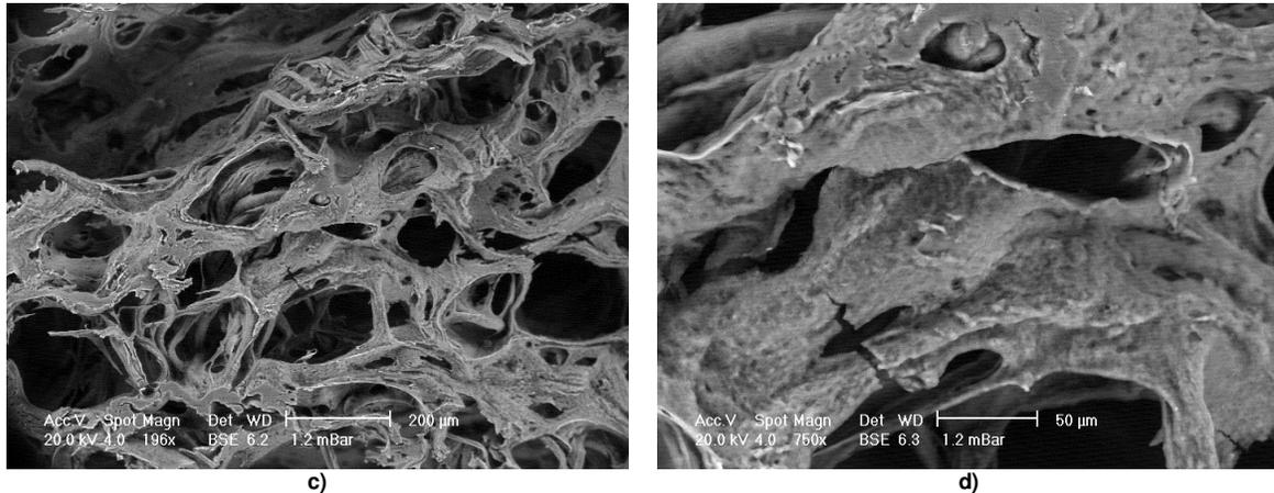
**Sponges made from the NaOH process: 5B389 cellulose/7.6NaOH/water with 2 reinforcing fluff fibres pre-impregnated with 8%NaOH/water at -6 $^{\circ}$ C, porophores added, 20 hours of freezing at -20 $^{\circ}$ C, regeneration in water at +70 $^{\circ}$ C**
