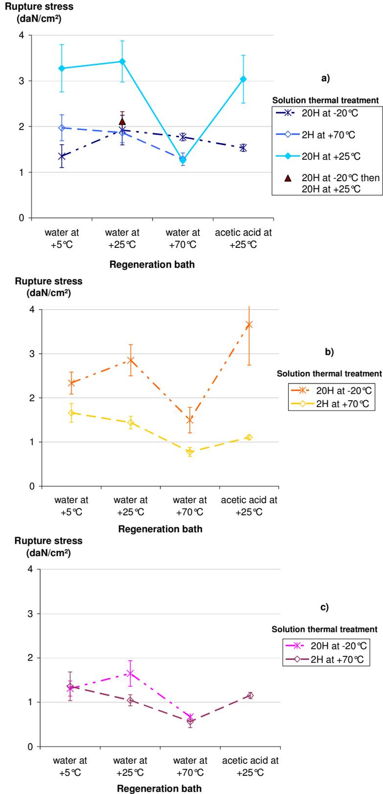
**Fig.V.2-2: Rupture stress of wet regenerated B407 cellulose for different solutions, treatments, regenerating baths**
