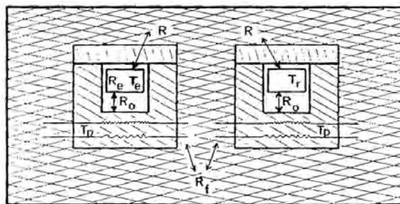
Fig.II.3-3: Various thermal resistances present in DSC
