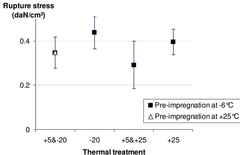
**Fig.V.2-8: Rupture stress for wet regenerated samples (in water at +70°C) as a function of thermal treatment for 5B389 cellulose/7.6NaOH/water+2 fluff pre-impregnated in 8%NaOH at +25°C ( $\Delta$ , one value at '+5&-20') and at -6°C ( $\blacksquare$ )**
