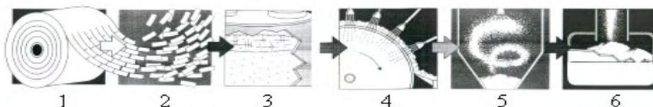
**Fig.I.1-8: Process to obtain microcrystalline cellulose**
