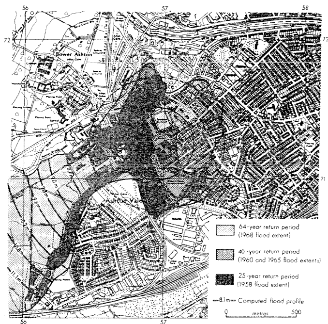
Fig. 8.4 Generalised flood profile and simulated flood extents
