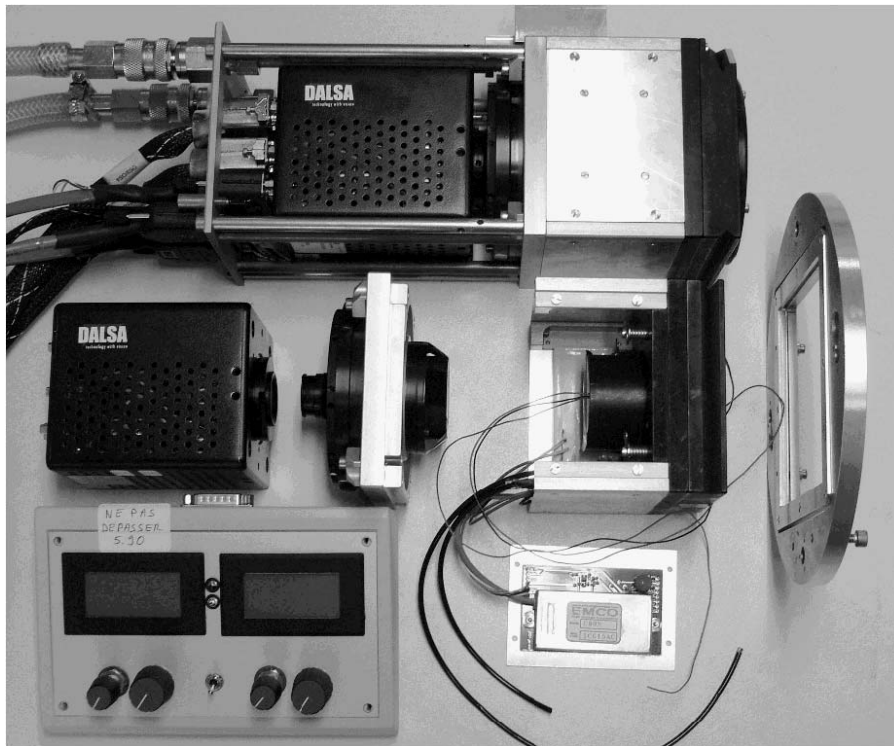
Figure 1. A CPNG camera and the elements of a second one. From right to left: fixation, image intensifiers, coupling lens, CCD camera. The intensifiers manual gain control is also shown.
