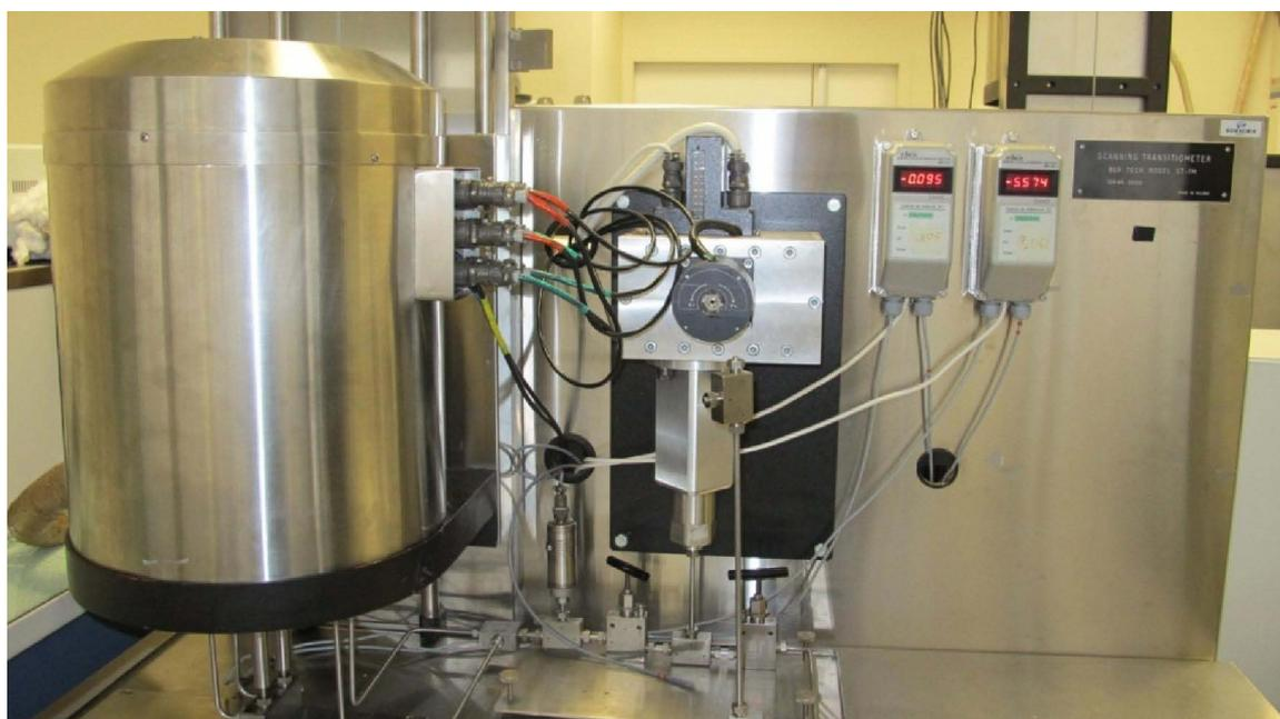
Fig. 2.4. Photo of transitiometer ST-7M.
