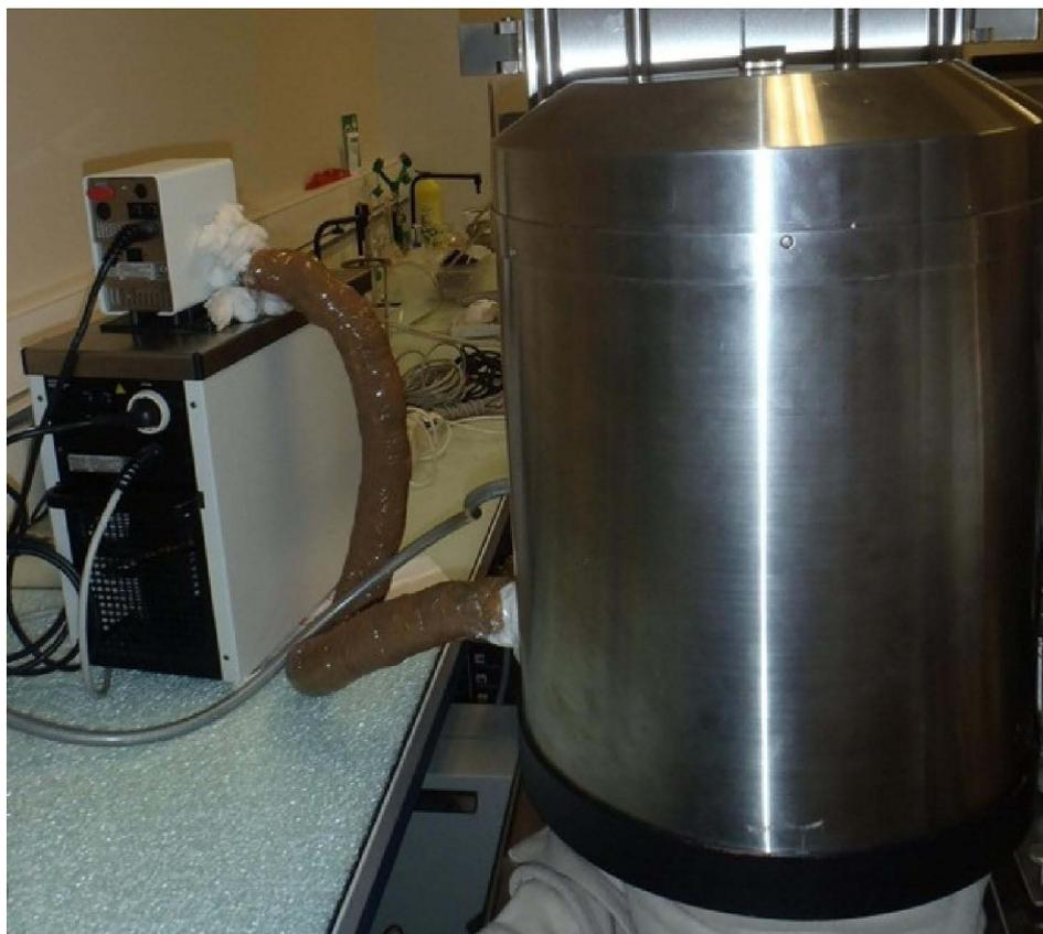
Fig. 2.7. Cryostat Thermo Haake K20 connected to transiometer ST-7M.
