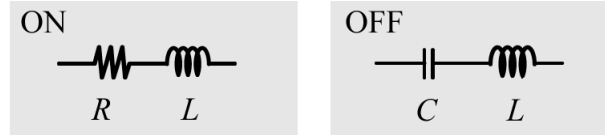
Figure 4.13.: p-i-n diode circuits equivalent
