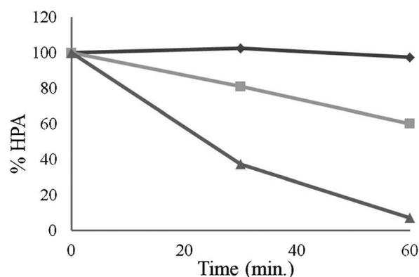
**Figure 6.** Li-HPA stability (50 mM = 100%) against time and temperature with mTK<sub>gst</sub>, ThDP and MgCl<sub>2</sub> in glycyglycine buffer. at 20°C ◆, 50°C ■ and 70°C ▲.
