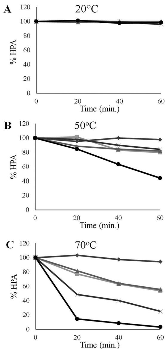
**Figure 5.** Li-HPA stability against time and temperature in the absence of TK in H<sub>2</sub>O ♦, in glycylglycine buffer ▲, in TEA buffer ■, in KH<sub>2</sub>PO<sub>4</sub> buffer ×, and in Hepes buffer ●. (A) Stability of Li-HPA at 20 °C, (B) at 50 °C and (C) at 70 °C. Li-HPA concentrations (50 mM = 100%) determined against time from aliquots of medium in the presence of L-lactate dehydrogenase as auxiliary enzyme and NADH by spectrophotometry at 340 nm.
