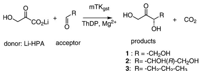
**Scheme 4.** Irreversible reaction catalyzed by mTK<sub>gst</sub> in the presence of hydroxypyruvate lithium salt (Li-HPA) as donor substrate and  $\alpha$ -hydroxy aldehydes (glycolaldehyde, D-glyceraldehyde) and generic butanal as acceptor substrates.
