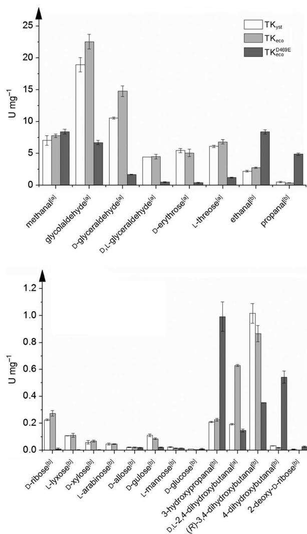
**Figure 4.** Determination of TK acceptor specificity. The assay solution contained [a] 50 or [b] 200 mM acceptor, 4, 12, or 32  $\mu\text{g}$  TK, 2.4 mM TPP, 9 mM  $\text{MgCl}_2$ , 0.028 mM phenol red and 2 mM TEA (pH 7.5). The reaction started after the addition of 50 mM LiHPA; total assay volume was 200  $\mu\text{L}$ . The OD increase was measured at 560 nm by a plate reader.
