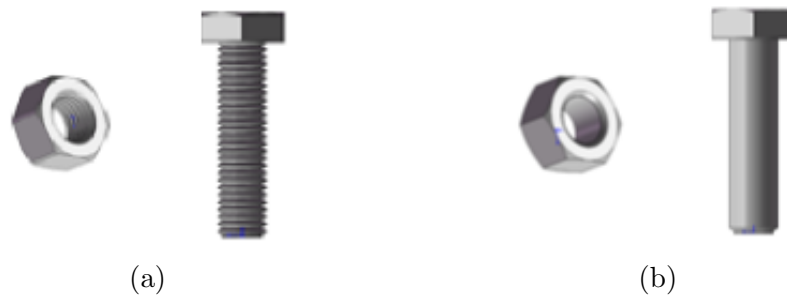
Figure 1.17: Screw and nut (a) in real configuration, (b) as simplified geometric model.
