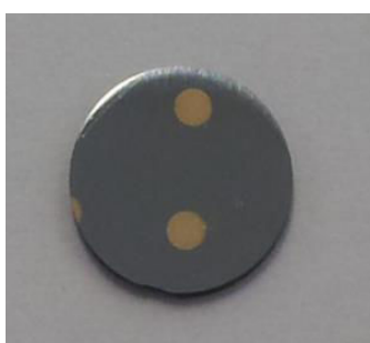
Figure 4-9 Photograph of a sample with two contacts for I-V measurements
