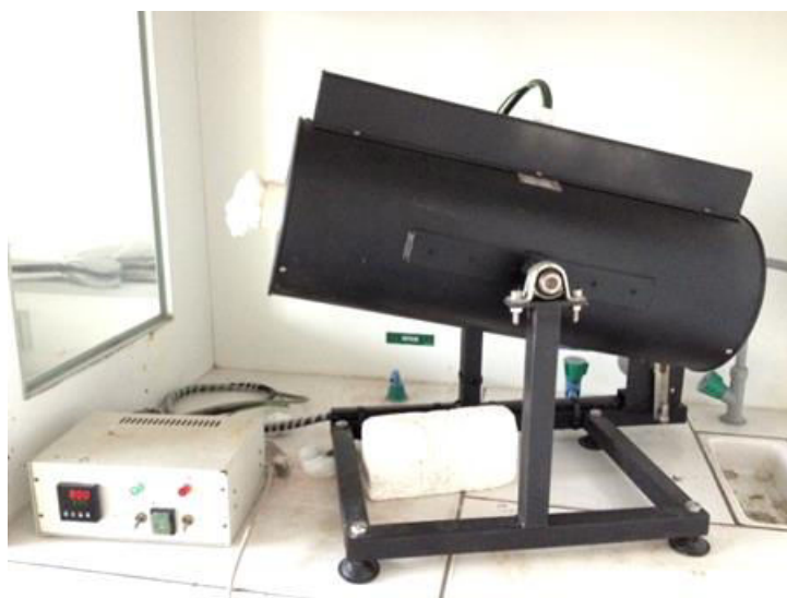
Figure 2-5 Photograph of a rocking furnace
