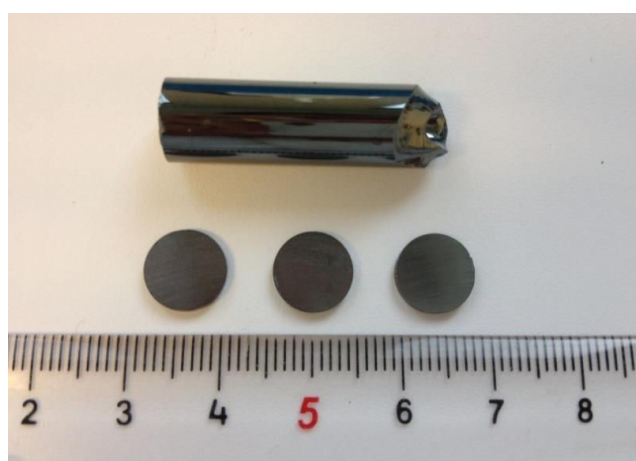
Figure 2-7 Photograph of glass rod and discs
