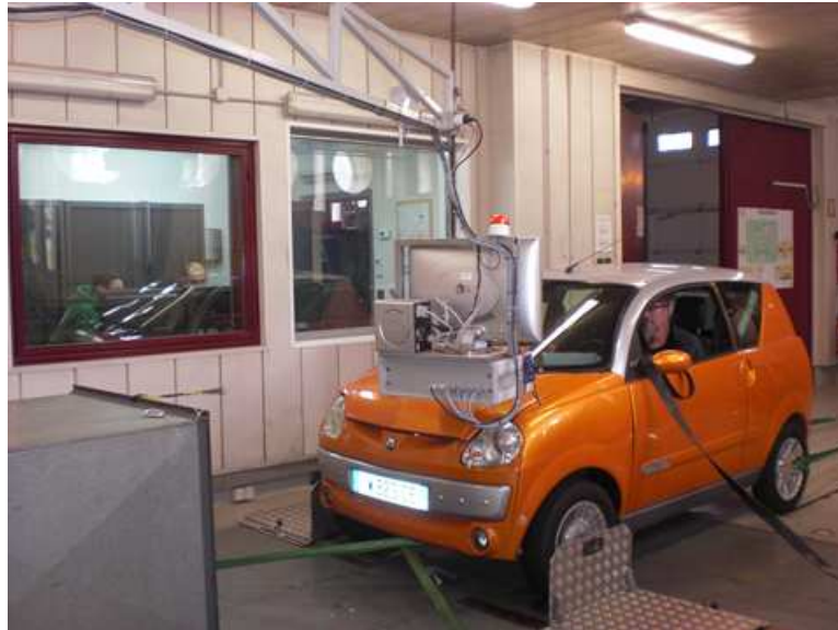
FIGURE 5.13: Chassis test bench
