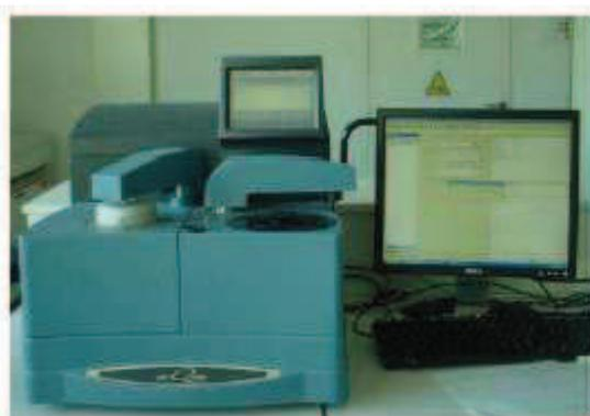
Figure 1. Appareil DSC Q2000
