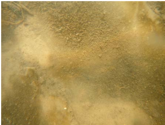
MR2_A (dst. RD 3,5m) D_{50}=52\mu\text{m}
