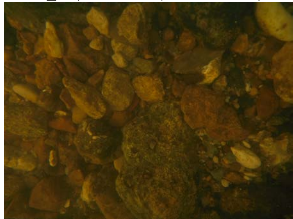
MR5_C (dst. RD 8m) D_{50} = 5\,301\mu\text{m}
