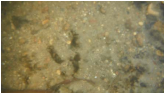
MR5_C (dst. RD 8m) D_{50} = 3\,207\mu\text{m}
