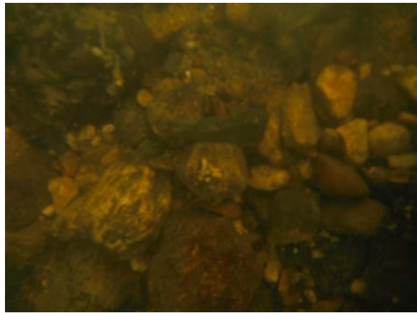
MR5_B (dst. RD 6m) D_{50} = 58\,012\mu\text{m}
