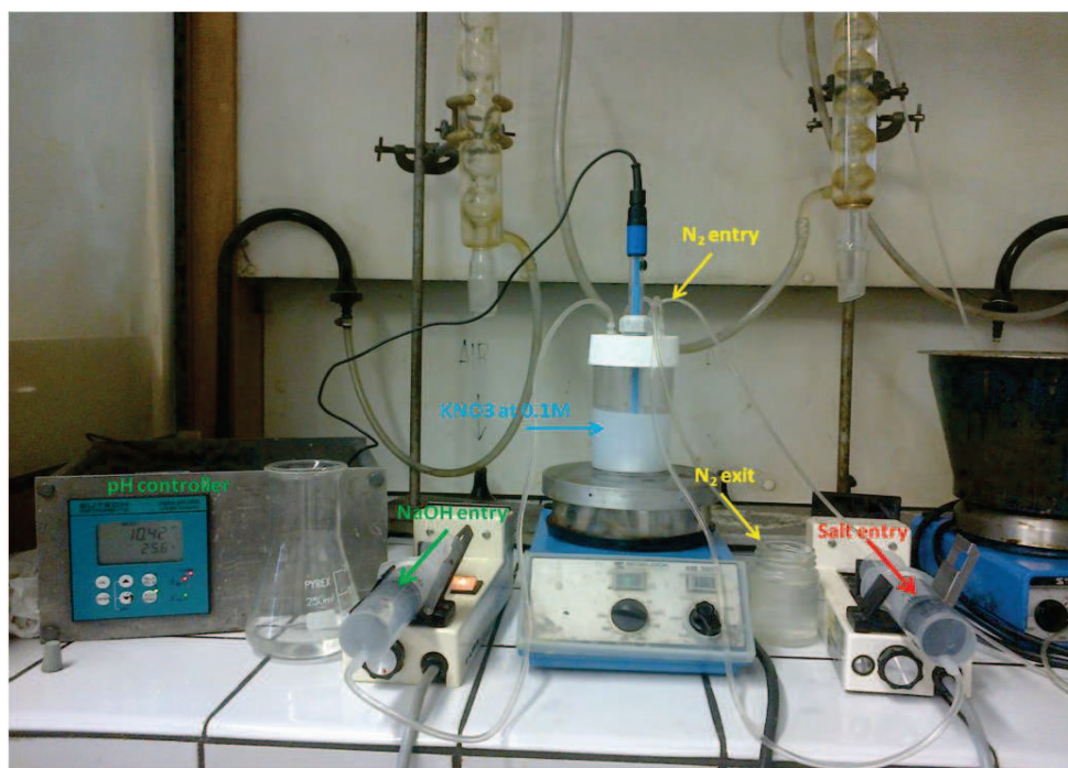
Figure 13. Typical system used to perform the direct coprecipitation of metallic salts for the synthesis of LDH phases.
