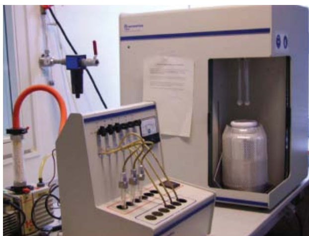
Figure 2.3 The Tristar Micromeritics sorptometer at ICPEES in University of Strasbourg. The machine on the left side is for the degas of samples which is possible for six samples simultaneously degass. The machine on the right side is for the analysis of the porosity, which can detect three samples ensemble.
