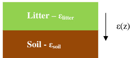
Figure 3.13: representation of the soil and litter layers as an effective medium with an effective permittivity that varies with depth z
