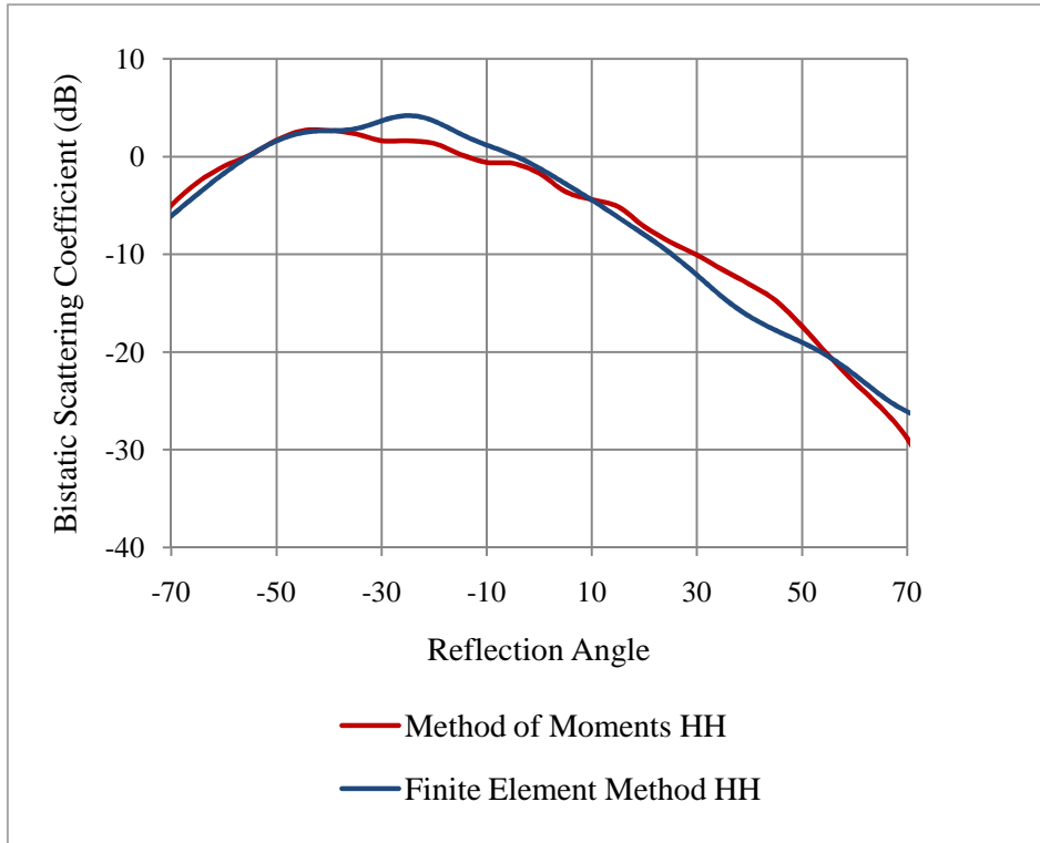
Figure 5.4: Bistatic scattering coefficient for the Method of Moments and the Finite Element Method models, calculated at 1.4 GHz for \epsilon_r=4+1i and [\sigma, L_c]= [3.41cm, 20.5cm] with an incident angle of 30^\circ and at polarization HH
