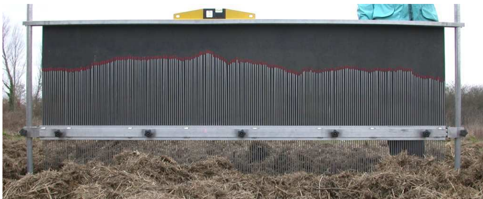
Figure 5.8: The needle board that was used to capture roughness profiles. The roughness profile is given by joining the red marks at the tops of the needles. Note that this particular profile was not taken for the 2006 campaign, but for a later campaign involving a vegetation cover. In the 2006 campaign the soil was bare.
