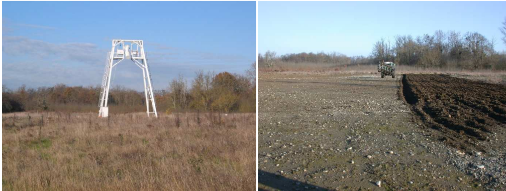
Figure 5.7: The LEWIS radiometer mounted on a tower, on the SMOSREX site, left and the soil being ploughed to create a rough surface, right.
