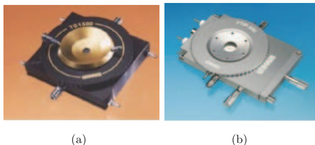
FIGURE C.2 – Images des fours Linkam : (a) LINKAM TS 1500. (b) LINKAM TMS 600.
