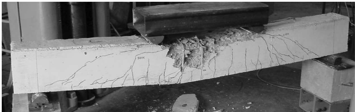
Figure I.2.24: Concrete crushing of FRP strengthened RC beam [Esfahania et al 2007].
