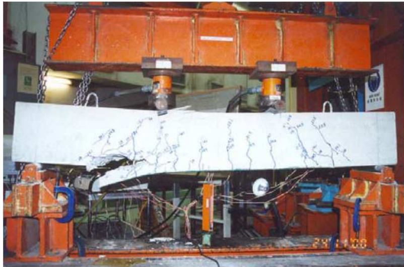
Figure I.2.35: FRP-plated RC beam: cover separation failure mode [Teng & Chen 2007].
