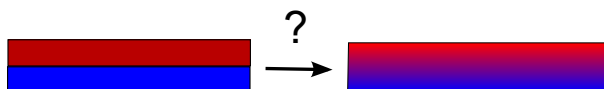
FIGURE 6.1 – Bi-layer system presented in Chapter 5 on the left compared to one with a continuous gradient discussed in this chapter
