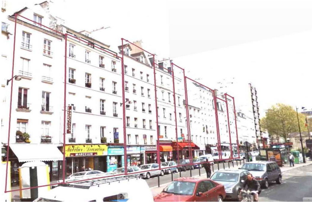
Figure 5.8: Estimated wire-frame model projected onto a panoramic image of the IGN Street Viewer.
