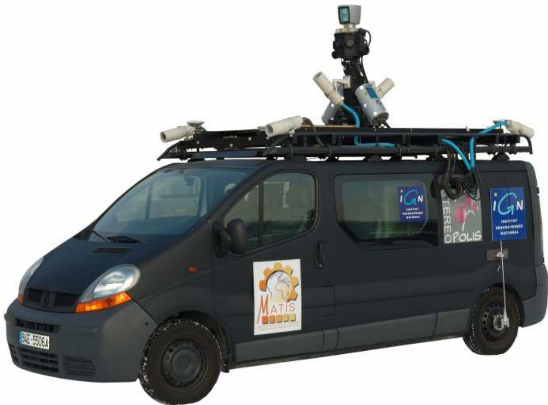
Figure 3.3: IGN Street Mobile Mapping System.
