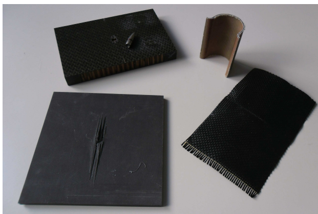
Examples of composite pieces: from raw fabric CFRP (bottom right) to impacted sandwich part (top left)
