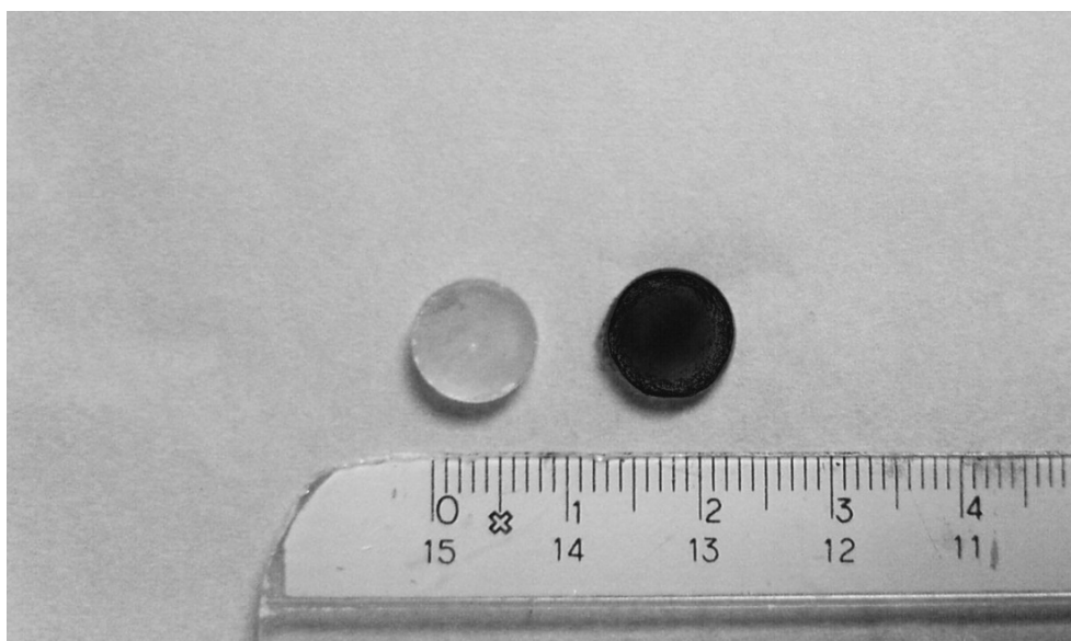
Figure IV. 5: The Von Kóssa reaction performed on the pellets: pellet of pHEMA remained translucent - left side; pellet of pHEMA-CM has strongly bound silver nitrate - right side
