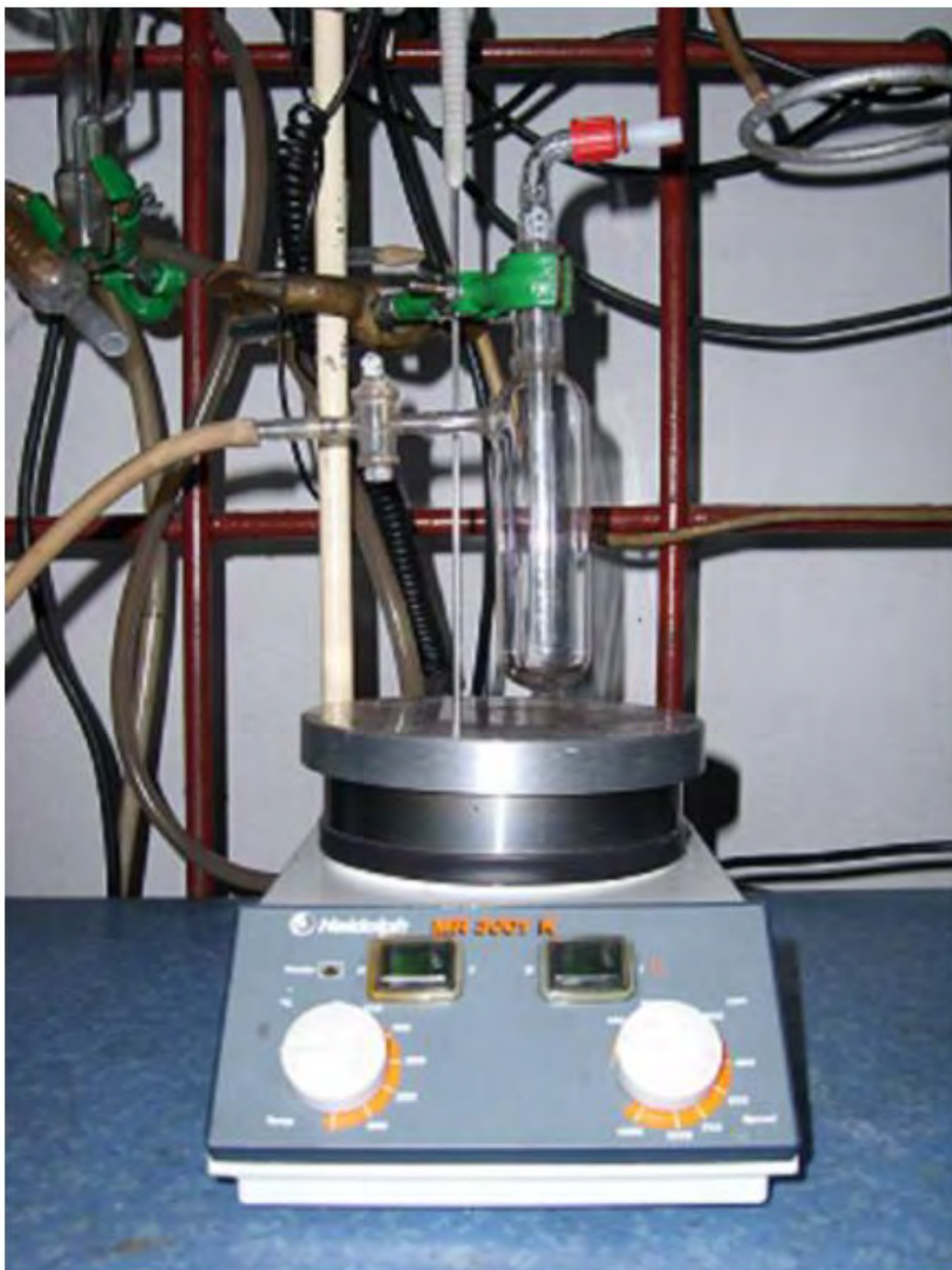
Figure III. 9: Lab installation for silk fibroin grafting monomer
