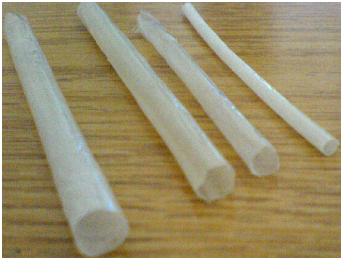
Figure II. 7: Image of four different diameter PHB tubes obtained by dry spinning method
