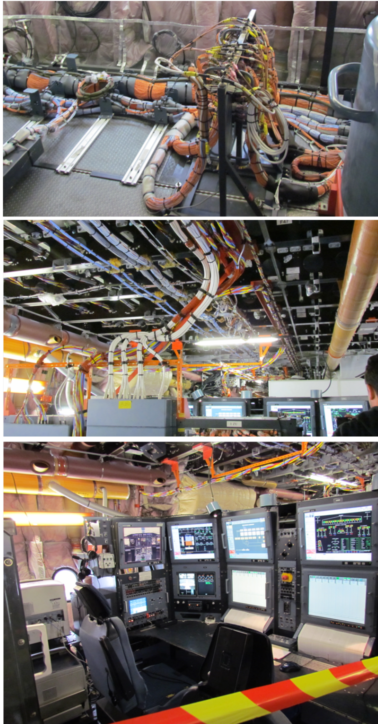
Figure 4: Equipments used to monitoring the Airbus A380 aircraft during test flights. http://www.flickr.com/photos/spacemike/6173378635/in/photostream/
