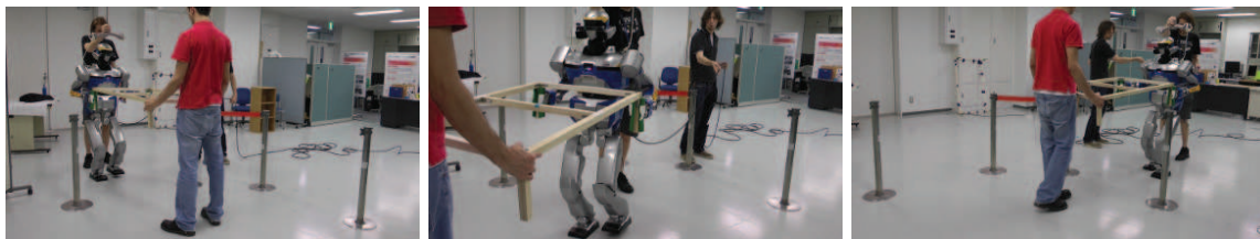
Figure 4.1: The task to perform: The human-robot dyad carries the beam through two doorways that form a 90^\circ angle. The dimensions of the beam do not allow performing the task with a single bend, so that the human has to pass backward through the first door and forward through the second one (and vice versa for the humanoid robot). The first picture (left) shows the starting position, whereas the last one (right) shows the stop condition when half the beam crosses the second doorway.
