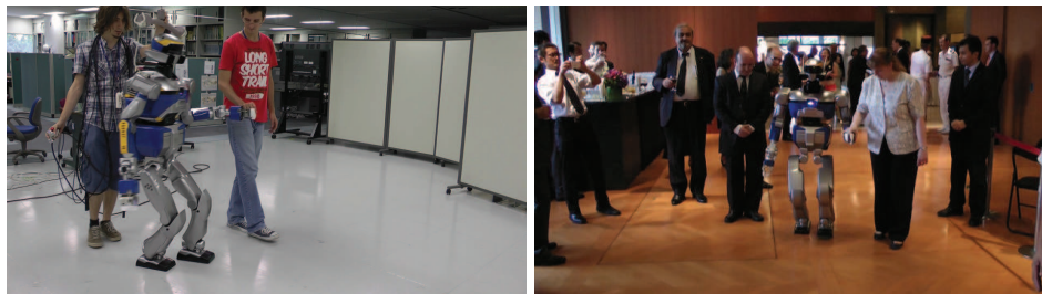
Figure 5.36: HRP-2 being guided by the hand in a lab environment (left) and at the French Embassy in Japan on July 14th 2012 (right).
