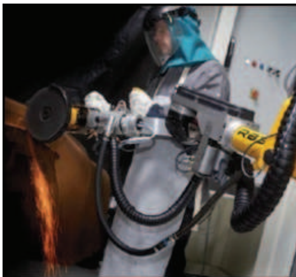
Figure 1.2: Cobot A7-15 is a collaborative robot that allows reducing the arduousness and the risks for operators in difficult manual tasks.
