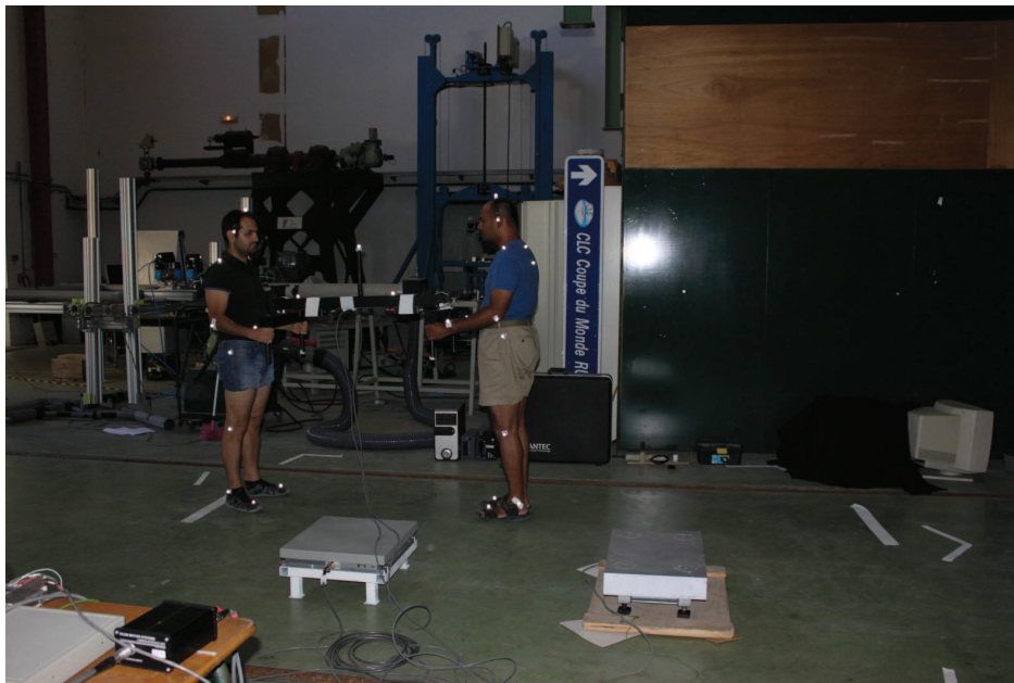
Figure 2.4: Experimental setup. The operational volume is a rectangular parallelepiped (4m long, 3m large and 2m high). The operational volume is separated in two zones: one with force plates in the foreground, one for the locomotion task in the background.
