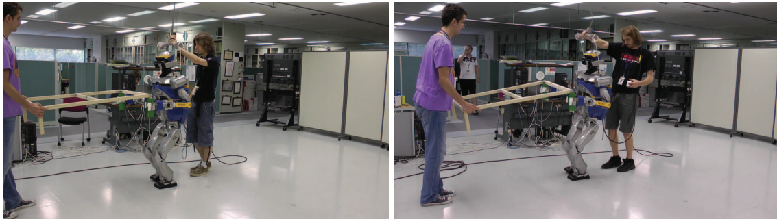
Figure 5.26: Test scenario with the stabilizer on (left) and off (right). The robot remains straight with the stabilizer on while it is leaning dangerously without it. The operator behind the robot has to assist in stabilizing the robot by stretching the ropes that are holding the robot in case it is falling.
