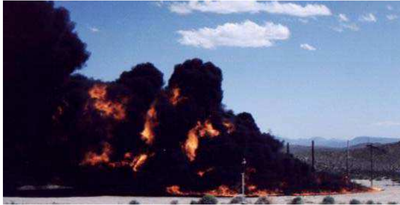
Figure IV.18 Instantaneous view of the experiment flame and smoke from a video camera for medium wind ( U_0=5.4 m/s)
