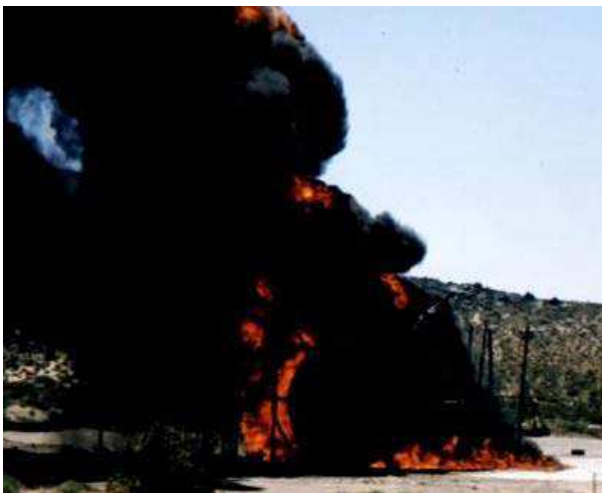
Figure IV.15 Instantaneous view of the experiment flame and smoke from a video camera for low wind ( U_0=1.9 m/s)
