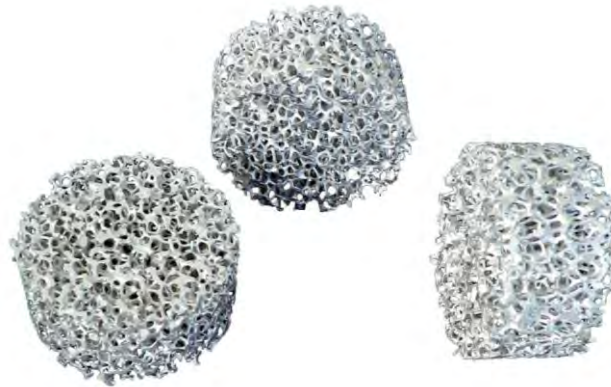
Figure 2.6: Example of Aluminium foam (ERG Duocel®).
