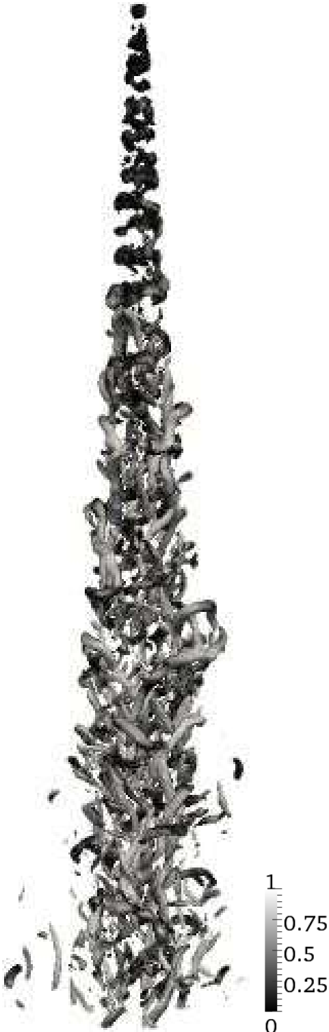
Figure 48: Iso-surfaces of Qn=0.25 colored by helicity
