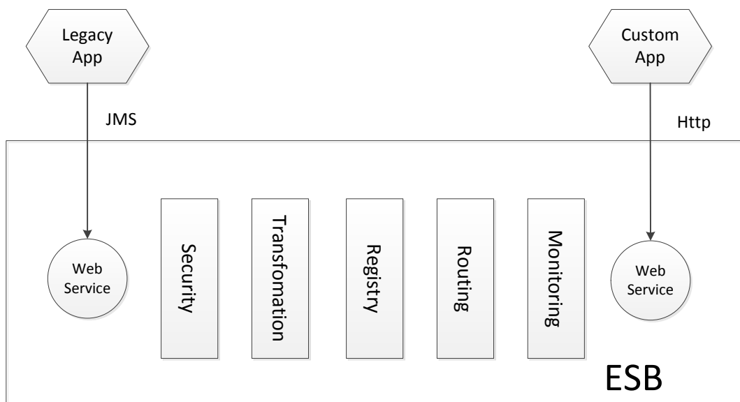
Figure.4.3 The basic structure of ESB (Image from (Bhat, 2008) )
